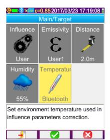
In case of Influence parameters, the measurements replace the user data entered in the Main/Target menu, provided that user influence is selected (see § 3.2.2. <u>Using the user compensation for the influencing factors</u>).
