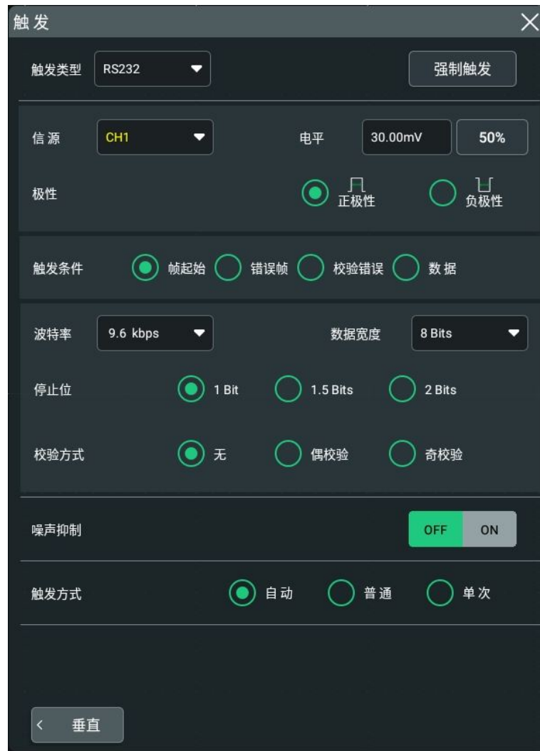
图 8.25 RS232 触发类型配置菜单
