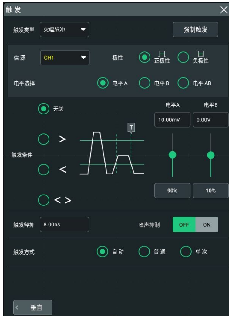
图 8.16 欠幅脉冲触发配置菜单
