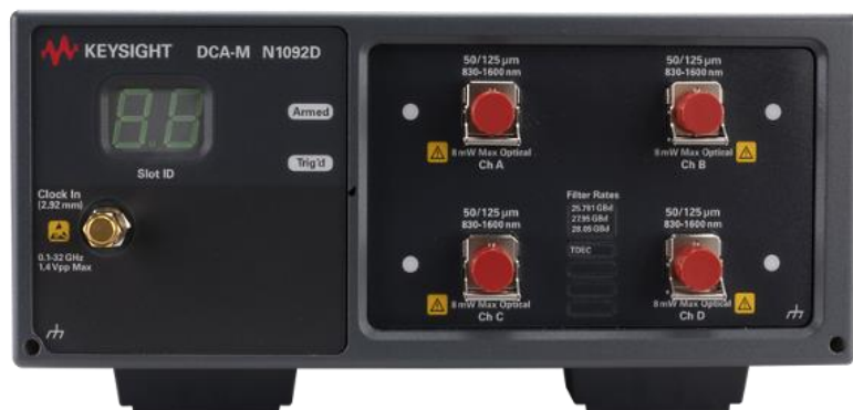
Figure 30. N1092D quad optical DCA-M with options 30A, 280 and 168
