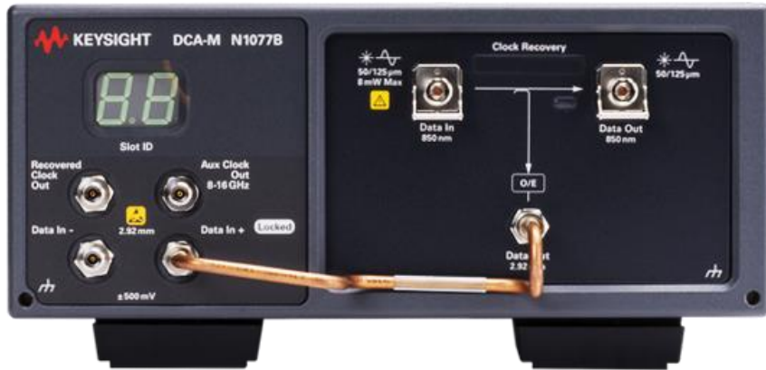
Figure 24. N1077B Multimode/Single-mode optical/electrical clock recovery with options 264 and SMM
