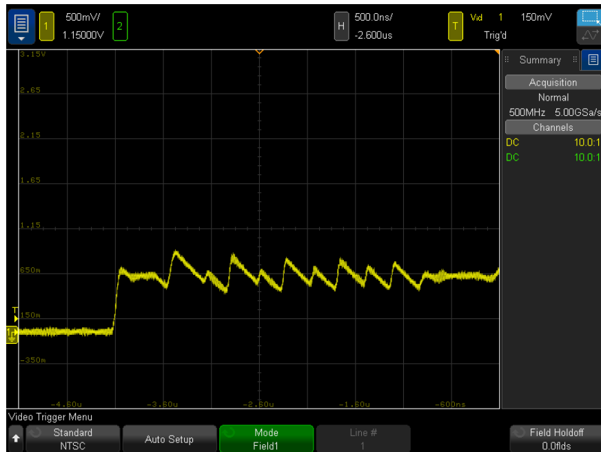
Figure 25 Triggering on Color Field 1 Alternating with Color Field 3
