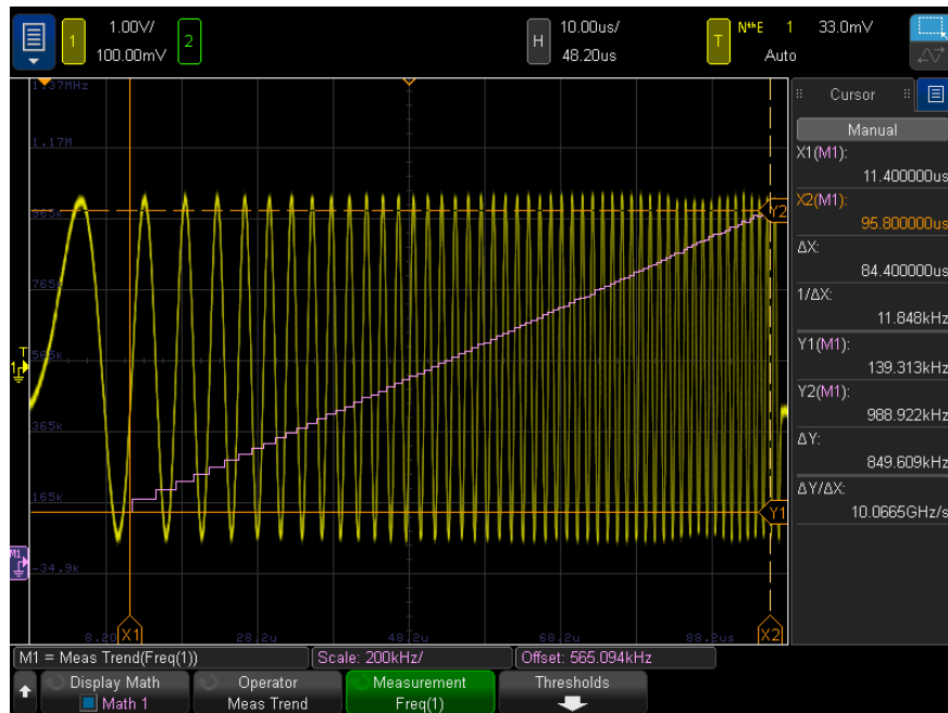
Figure 17 Example of Measurement Trend
