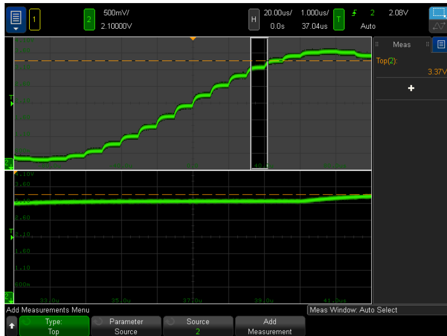
Figure 40 Isolating area for Top measurement
