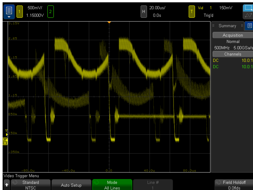
Figure 22 Triggering on All Lines
