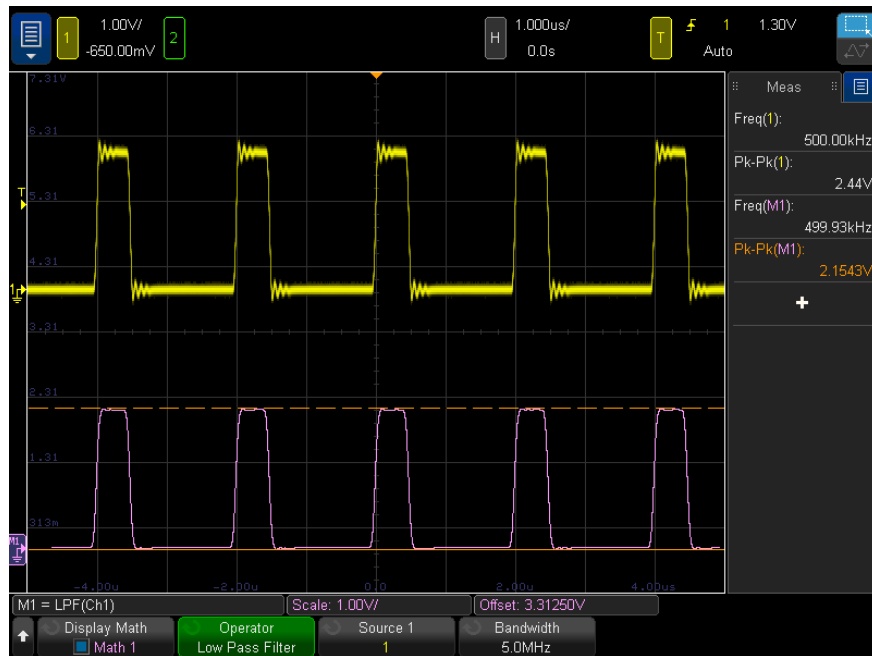
Figure 15 Example of Low Pass Filter
