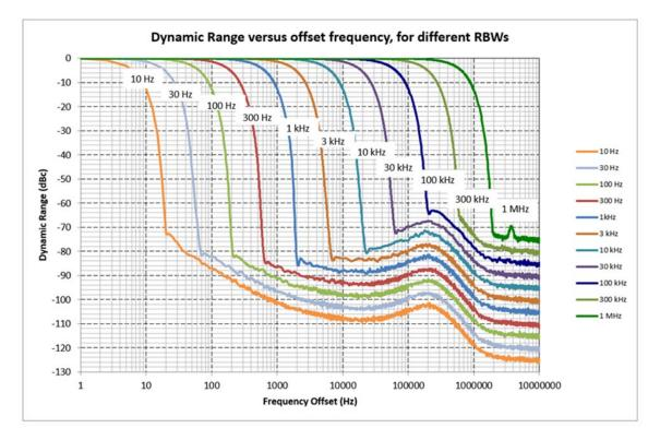
$<sup>^{1}</sup>$  For 1 MHz RBW, the sideband observed may degrade the dynamic range to -70 dBc
