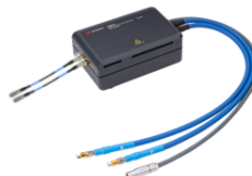
Figure 3. Four remote heads are available for the pattern generator module M8042A. At the top the 120 GBd remote heads M8059A and M8069A are shown with 1.0 mm connectors to accommodate close connection to the device under test for symbol rates up to 120 GBd. The 64 GBd remote heads M8058A and M8068A are shown at the bottom, these provide 1.85 mm connectors. The three cables on the back side of the remote heads are used to connect with the M8042A pattern generator module and are not removable.
