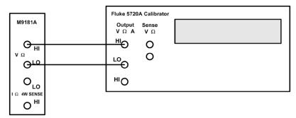
**3** Compare AC voltage measurement results from the M9181A DMM to the appropriate test limits shown in the table. Be certain to allow for appropriate source settling.
