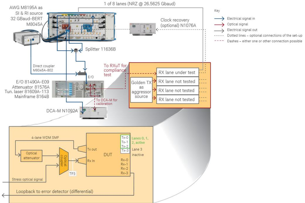
Figure 12 Optical receiver stress test setup for 200 GBASE-LR4/-FR4
