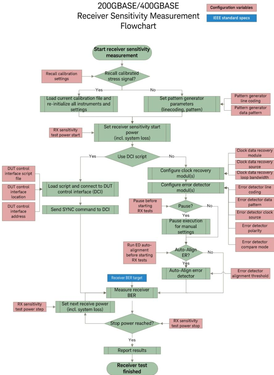
Figure 42 Receiver sensitivity measurement test procedure
