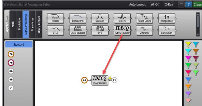
Figure 31 TDECQ operator dragged into the window's operator palette
