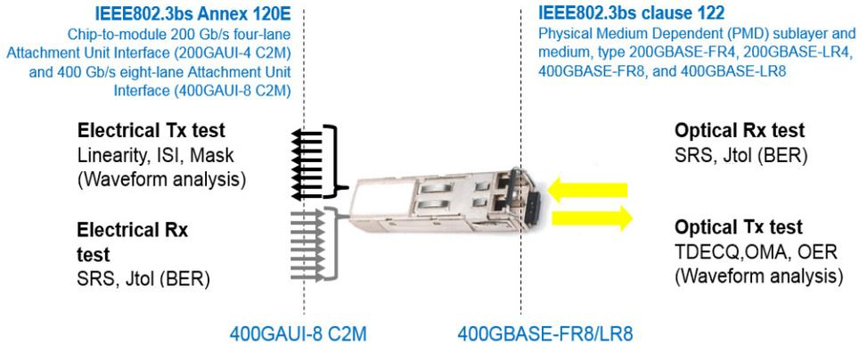
Figure 1 Overview of physical layer compliance tests for a typical 400GBASE-FR8 transceiver
