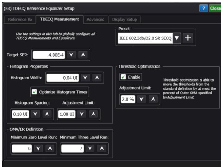
Figure 35 TDECQ Measurement tab with IEEE 802.3db/D2.0 SR SECQ preset
