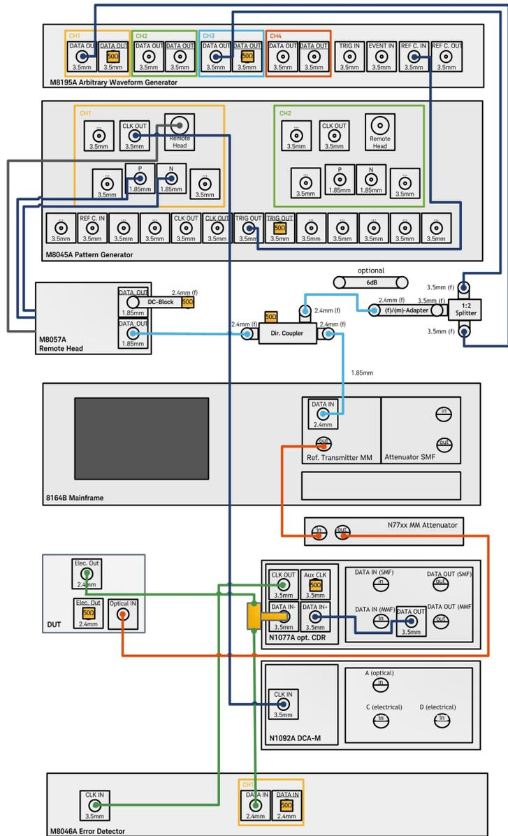
Figure 11 Setup for stressed eye signal calibration for 50G-SR/100G-SR2/200G-SR4/400G-SR8/100G-SR/200G-SR2/400G-SR4
