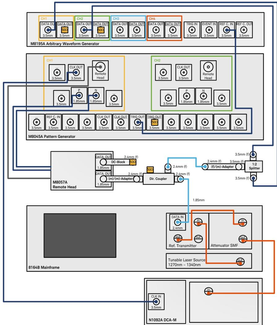
Figure 8 Setup for stressed eye signal calibration for 200GBASE-FR4/-LR4/-DR4 & 400 GBASE-FR8/LR8 with clean clock
