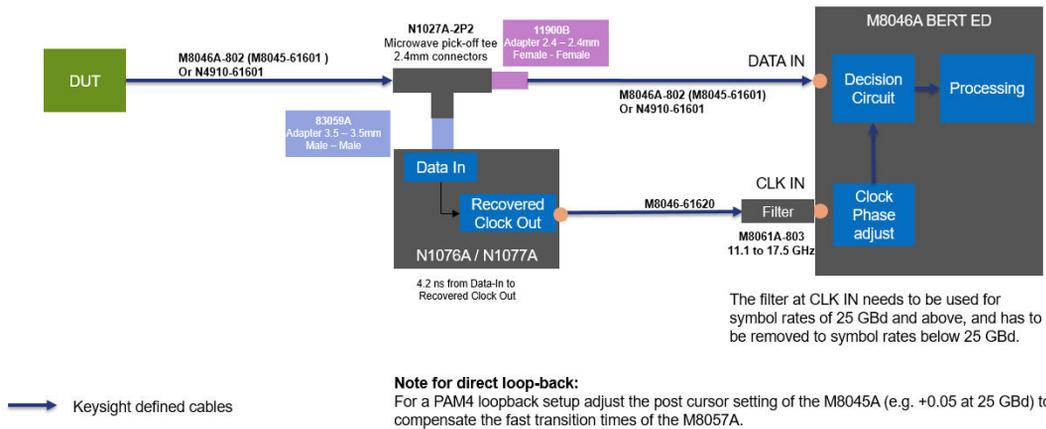
Figure 13 Recommended connection setup for N1076A/77A control
