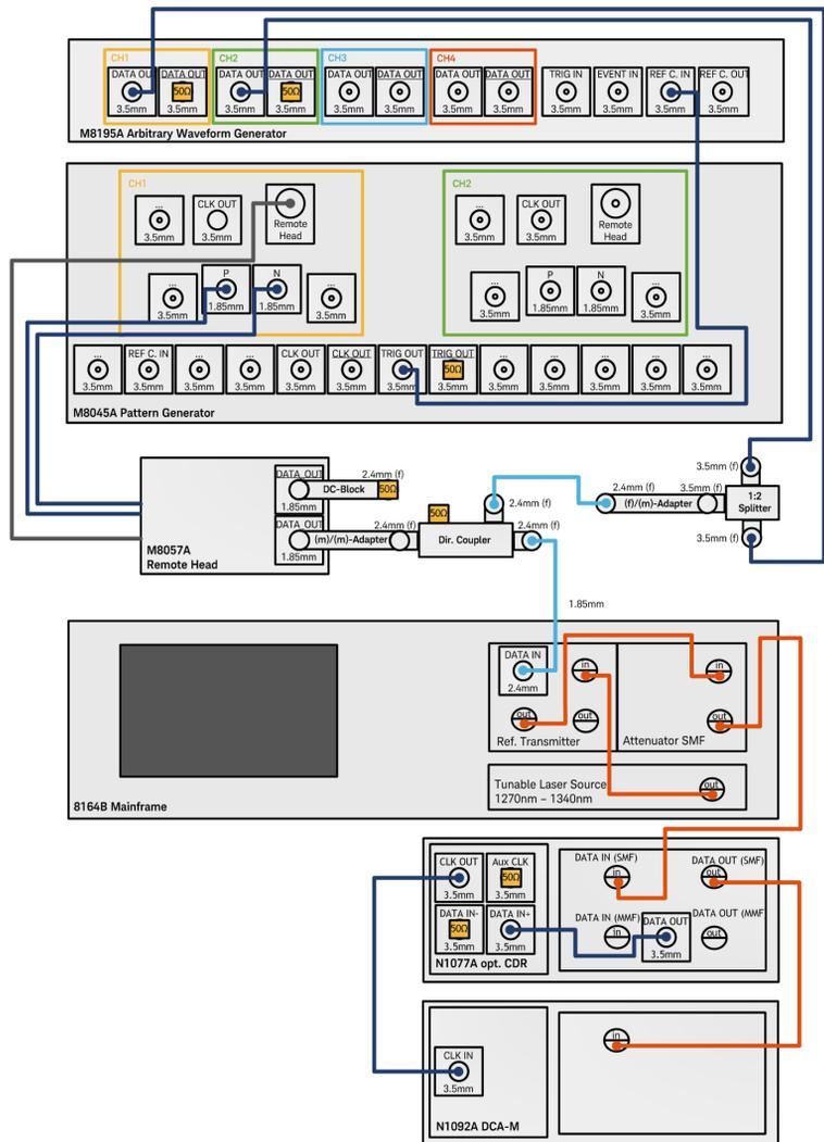
Figure 9 Setup for stressed eye signal calibration for 200 GBASE-FR4/-LR4/-DR4 & 400 GBASE-FR8/LR8 with recovered clock
