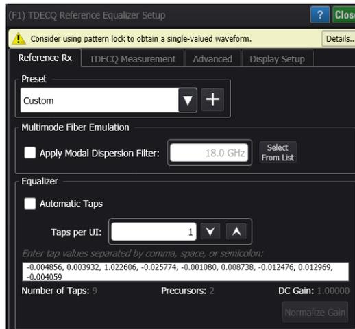
Figure 32 TDECQ Reference Equalizer Setup window
