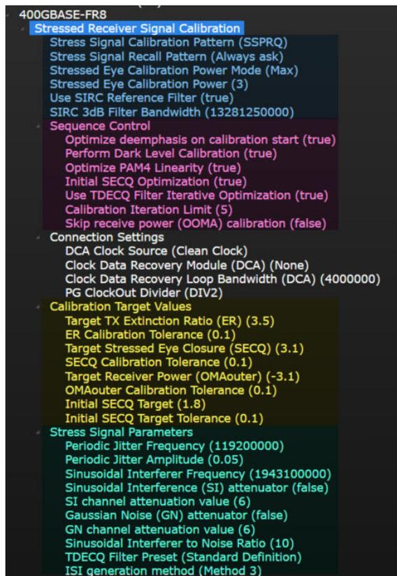
Figure 26 Exemplary stressed receiver signal calibration configuration variables for 400GBASE-FR8
