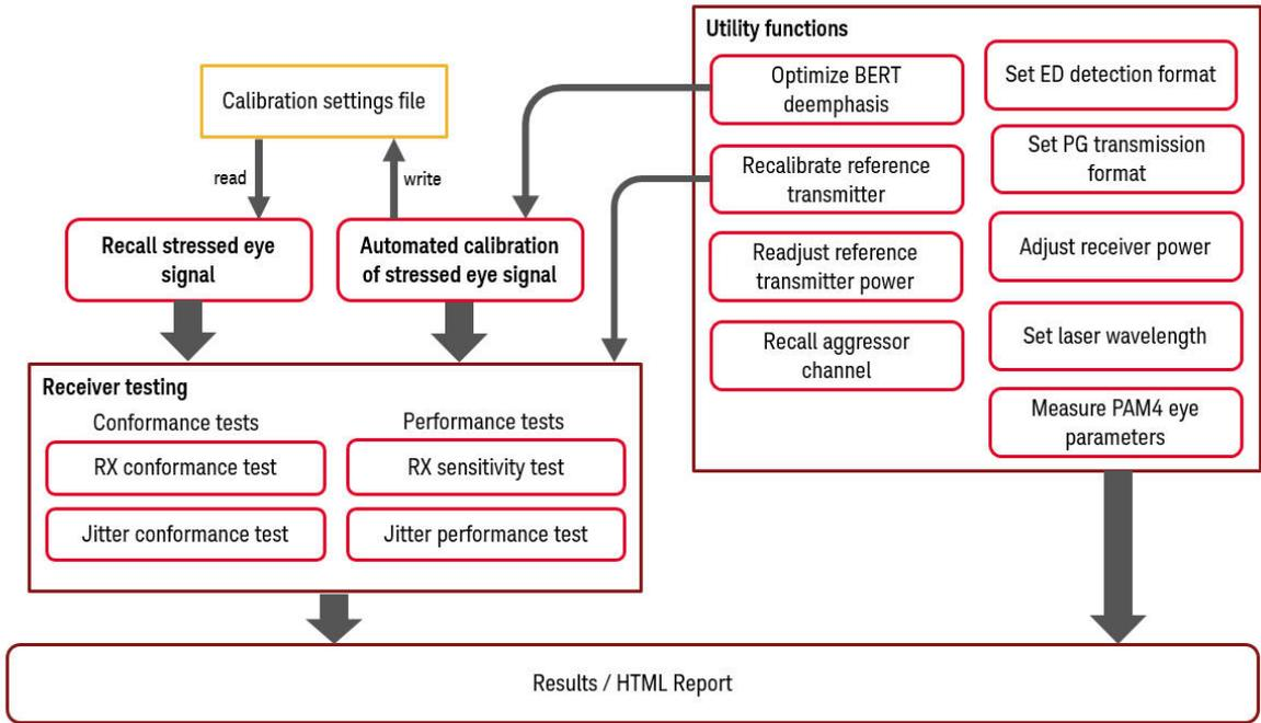
Figure 7 N4917BSCB Optical Receiver Testing Flow Chart
