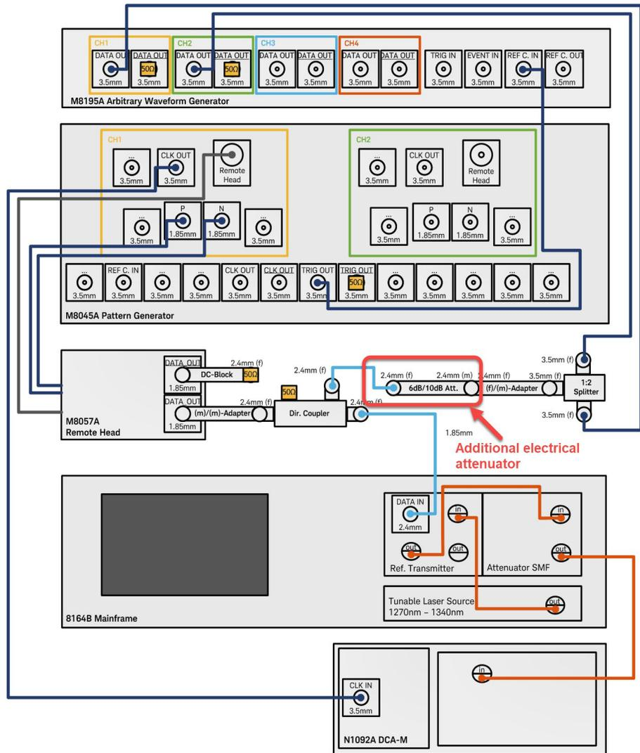
Figure 10 Setup for stressed eye signal calibration for 400GBASE-DR4 and 400G-FR4 (with additional electrical attenuator)
