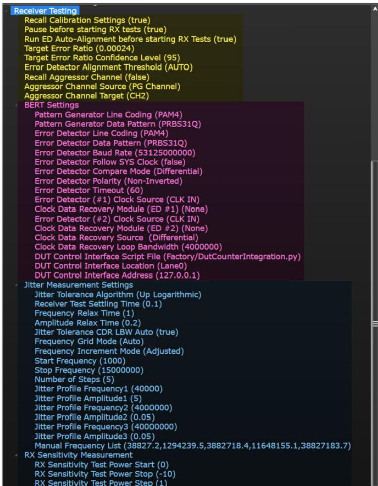
Figure 38 Configuration variables for receiver testing
