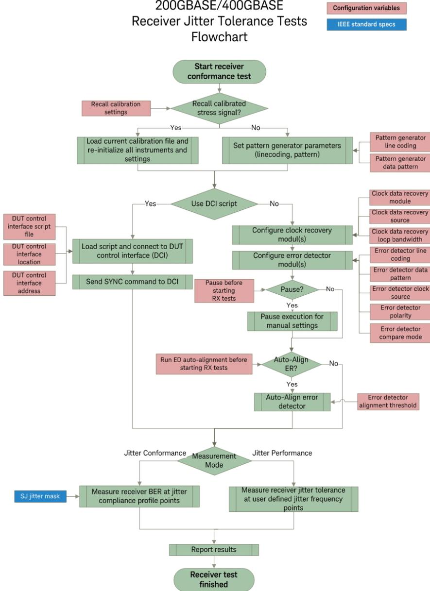
Figure 41 Receiver jitter tolerance tests procedure
