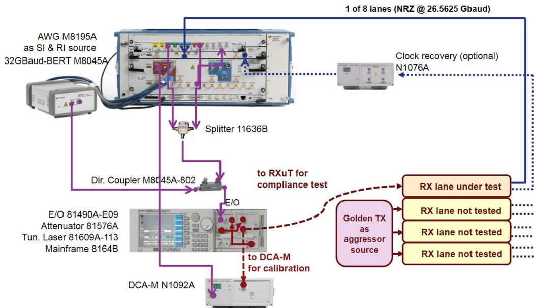
Figure 22 Equipment connections for IEEE802.3bs/cd calibrations and tests
