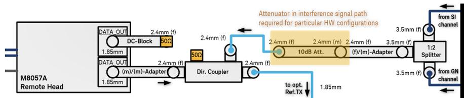
Figure 27 Placement of RF Attenuator
