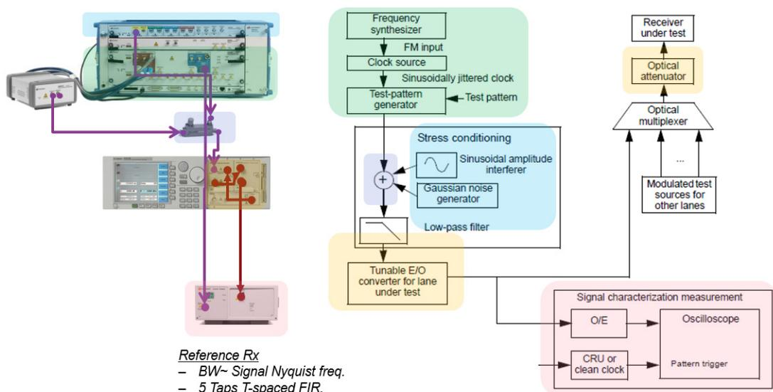
Figure 2 Stress receiver conformance test according to the IEEE and corresponding N4917BSCB equipment configuration
