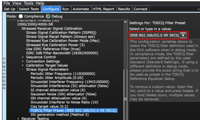
Figure 36 Manually selecting TDECQ Filter Preset in Debug mode
