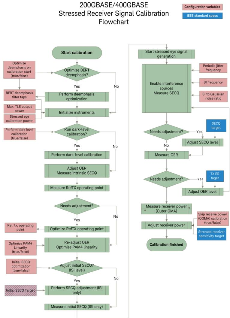
Figure 28 Stress signal calibration procedure
