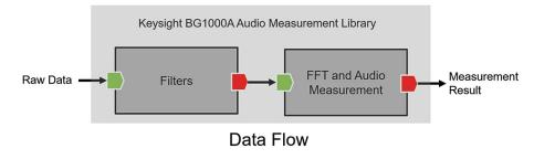
Figure 3. BG1000A data flow in an audio signal processing and analysis
