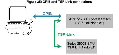
To configure the TSP-Link communication interface, each instrument must have a unique TSP-Link node number. Configure the node number for the Model 707B or 708B to 1 and the SourceMeter Instrument to 2.
