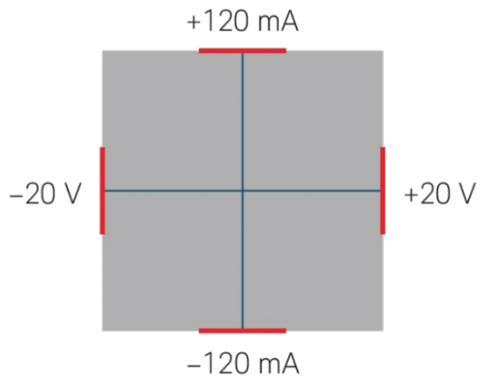
The U2722A/U2723A SMU is a versatile device that allows you to perform sweep and measurement from different operating regions without needing extra configurations. The four-quadrant operation
