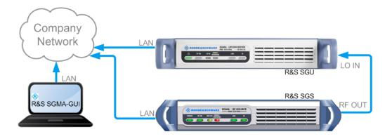
Figure 7-5: Connection of an R&S SGS and an R&S SGU in a company network
