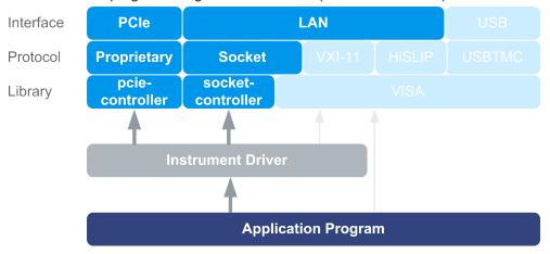
Figure 12-4: Remote control program using instrument driver (VISA not available)
