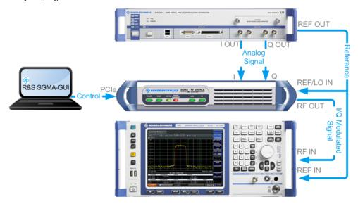
Figure 11-1: Example of the setup
