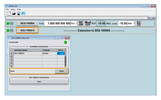
Connecting an R&S SGS and an R&S SGU
