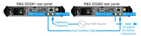
Figure 11-3: Example of a setup: LO coupling
