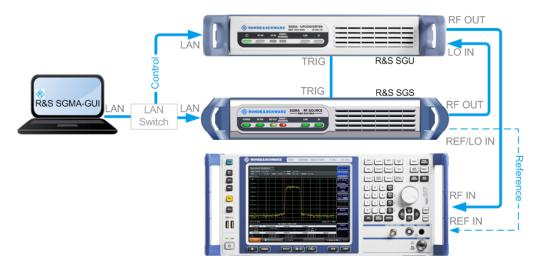
Figure 7-8: Example of a test setup for upconverting a CW signal generated by the R&S SGS
