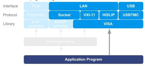
Figure 12-2: Remote control program using VISA
