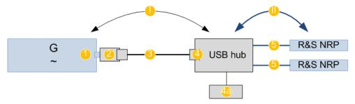
Figure 9-3: Connecting power sensors to the R&S SGS via USB hub
