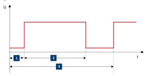
Figure 9-4: Pulse generator - single pulse mode
