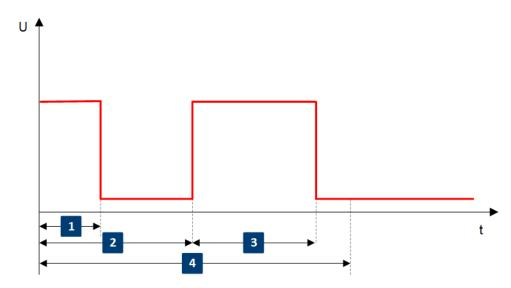
Figure 9-5: Pulse generator - double pulse mode
