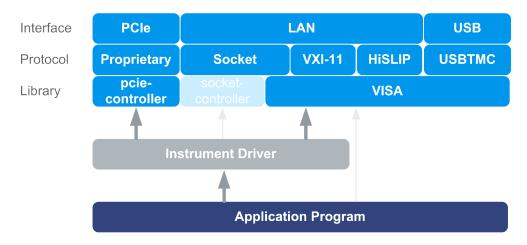
Figure 12-3: Remote control program using instrument driver (VISA available)
