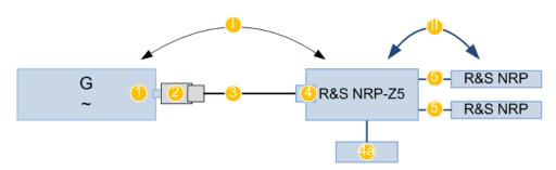
Figure 9-2: Connecting power sensors to the R&S SGS via R&S NRP-Z5 sensor hub
