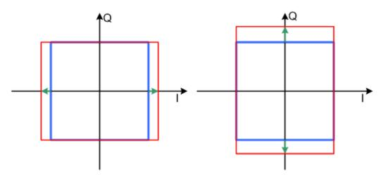
Figure 9-7: Negative gain imbalance (left) and positive (right) gain imbalance in the I/Q constellation diagram
