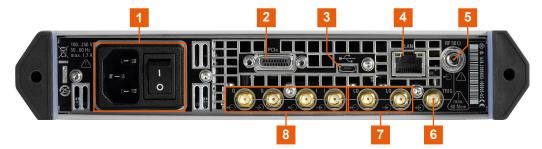
Figure 4-2: R&S SGU rear panel controls and connectors
