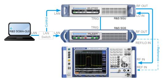
Figure 5-1: Example of a test setup for upconverting a CW signal generated by the R&S SGS
