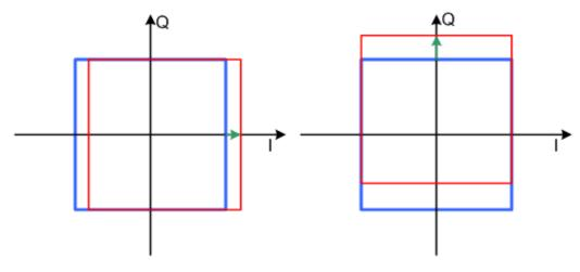
Figure 9-3: I offset (left) and Q offset (right) in the I/Q constellation diagram
