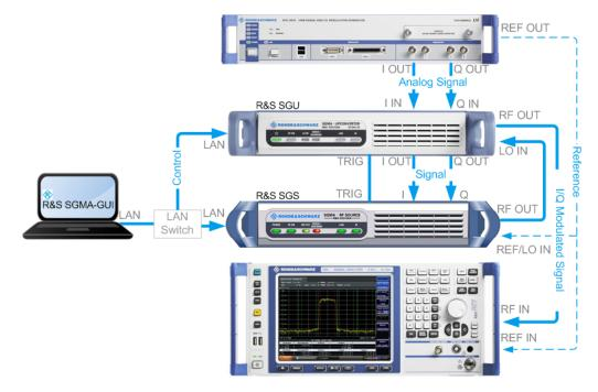
Figure 11-1: Example of the test setup
