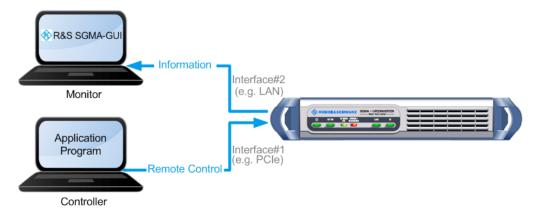
Figure 12-7: Example of a setup for remote control monitoring
