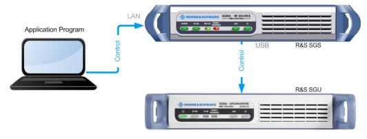
Figure 7-3: R&S SGU as an extension to an R&S SGS
