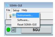
The setup menu provides access to dialogs for setting the general settings of the software, like dialogs for managing the connected instruments or dialogs providing information about the installed options.
