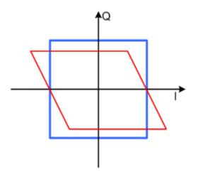
Figure 9-4: Positive quadrature offset in the I/Q constellation diagram
