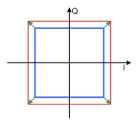
Figure 9-1: Effect of an increased amplitude in the I/Q constellation diagram
