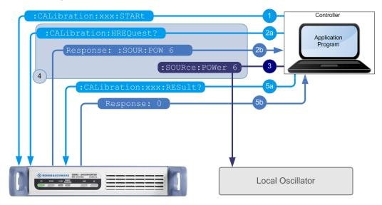
Figure 13-1: Calibration process of the R&S SGU. No physical connections between the instruments are shown in this graphic.
