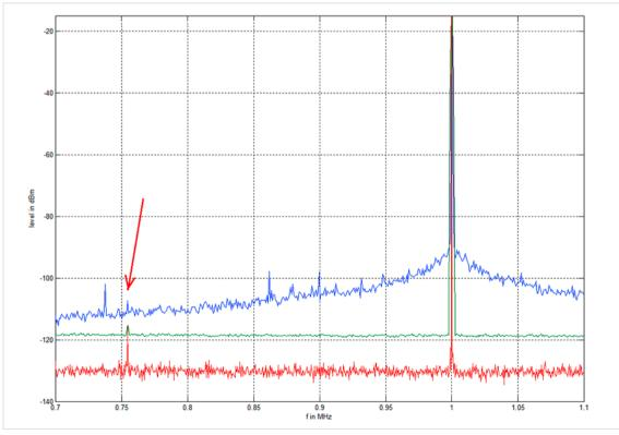
Blue: conventional analyzer with 10 kHz measurement bandwidth. Green: R&S\*FSWT with 10 Hz measurement bandwidth.
