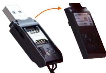
3. Insert the smart card with the chip facing downwards, and the angled corner (orange circle) facing away from the USB dongle:
