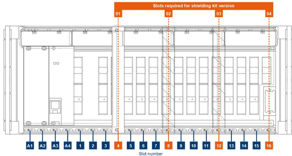
**Figure 3-3: Slot requirement for installation of shielding kit**
