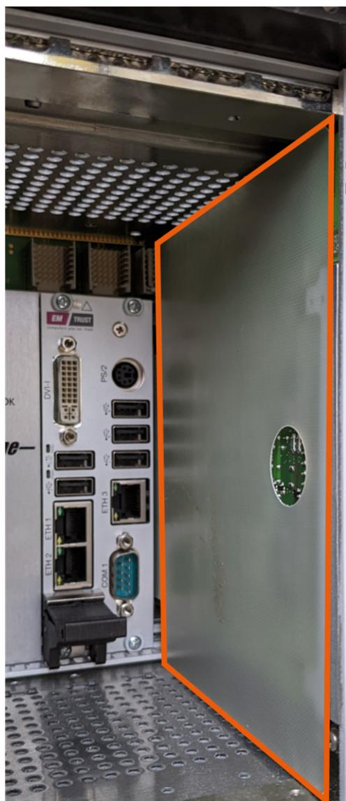
*Figure 3-7: Install insulation plate*
