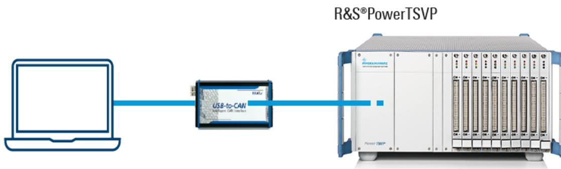
Figure 3-11: R&S PowerTSVP to external PC connection
