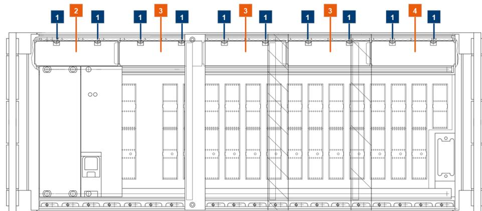
**Figure 3-4: Mount shielding kit covers (front view)**
