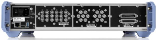
Rear view R&S®OSP220 and R&S®OSP230 units, rear module slots RS01 to RS03 (from left to right) with options
