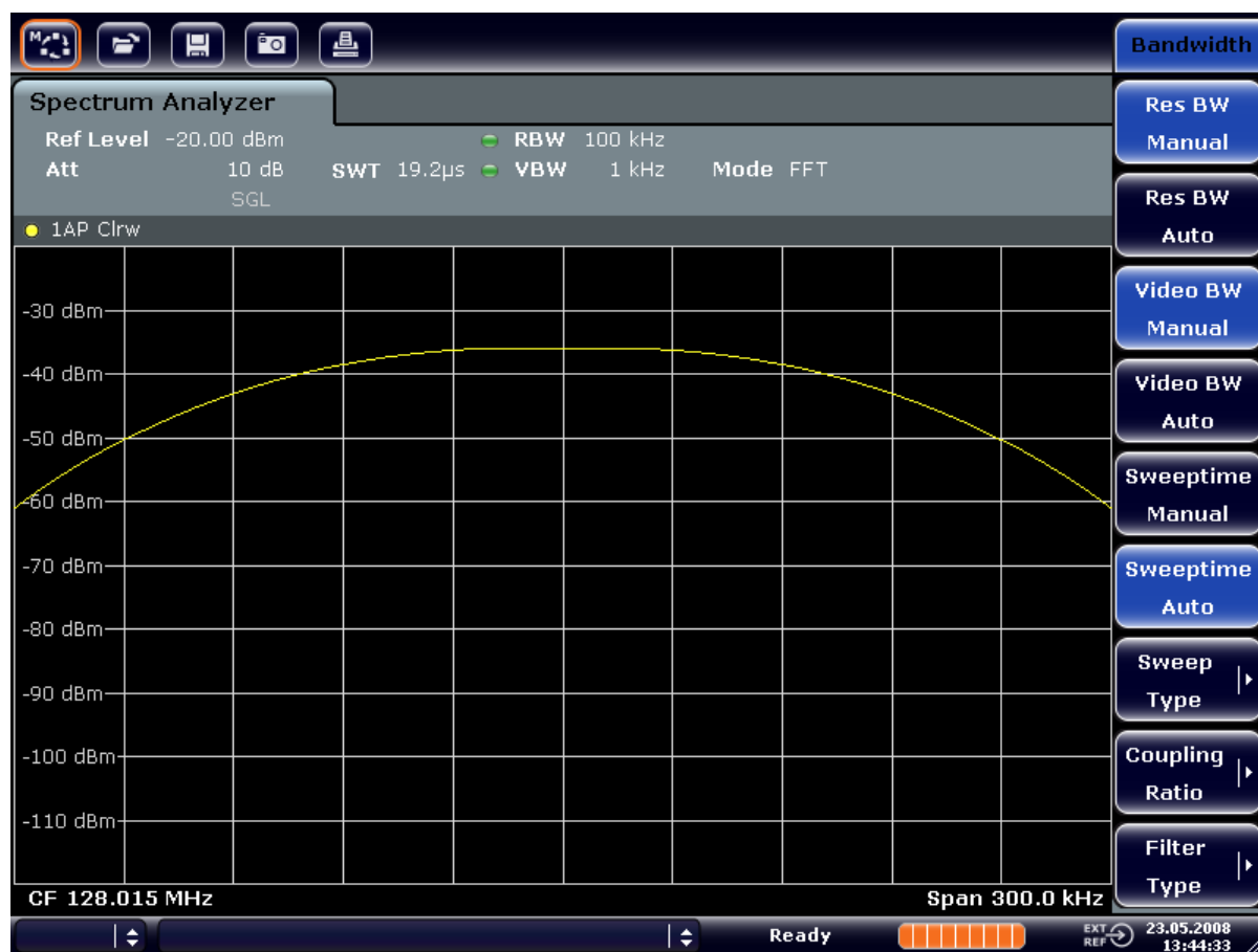
Figure 8-5: Measurement of two equally-leveled RF sinusoidal signals with a resolution bandwidth which is larger than their frequency spacing
