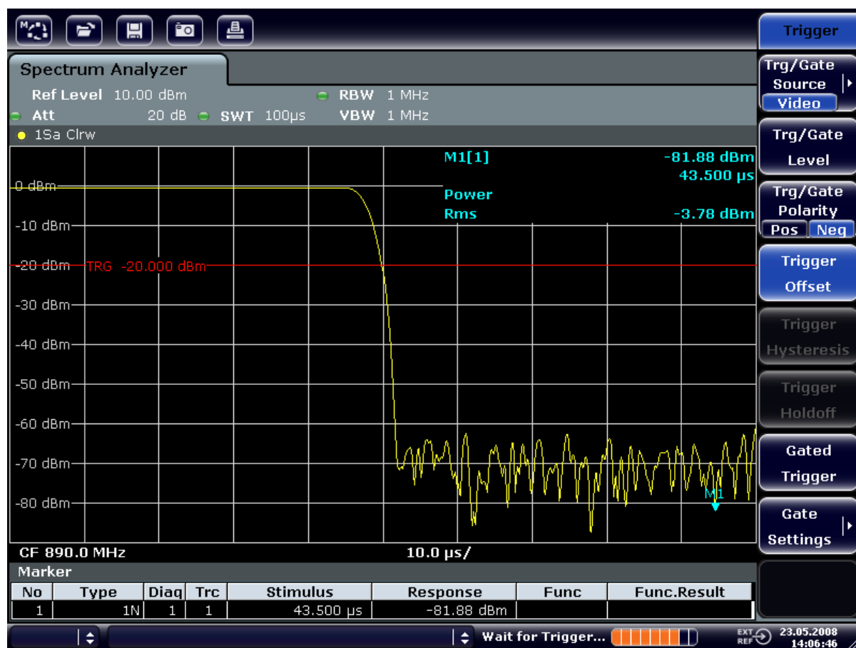
Figure 8-10: Falling edge of the GSM burst displayed with high time resolution
