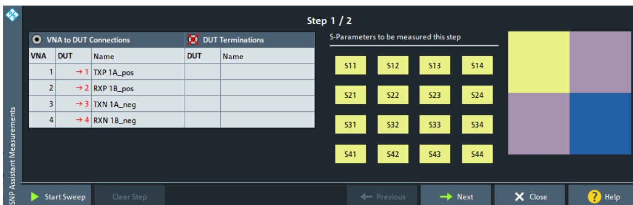
Figure 4-37: Step 3: Measure and/or import S-parameter data
