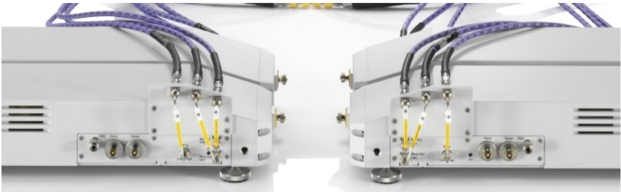
Figure 3-19: Standard arrangement for 4 external test sets
