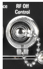
Figure 3-2: RF Off Control, terminated with attached Short
