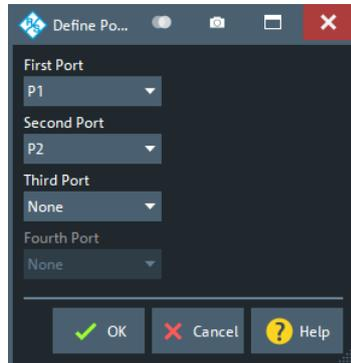
Use the controls on the right-hand side of the dialog to define the port set and the order of the ports within the port set.
