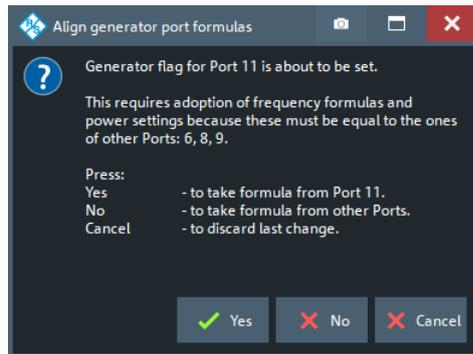
An **external generator** always represents a permanent signal source that is switched on for all partial measurements. "Source Gen" determines whether the generator is available as a signal source in the test setup. The analyzer provides two alternative, independent ways of selecting a generator as a signal source:
