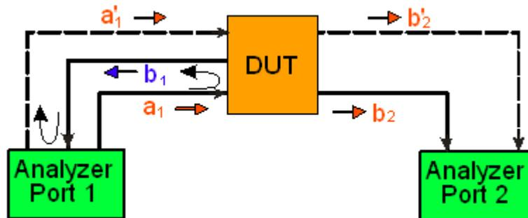
$LO > RF$  implies that  $LO = RF + IF$ . The mixer at port 2 converts both the wanted signal  $b_2$  and the spurious signal  $b'_2$  which is at the frequency  $RF' = IF + LO$ , to the same IF frequency. The response of an ideal, infinitely steep bandpass filter with a pass band between  $B^-$  and  $B^+$  looks as follows:
