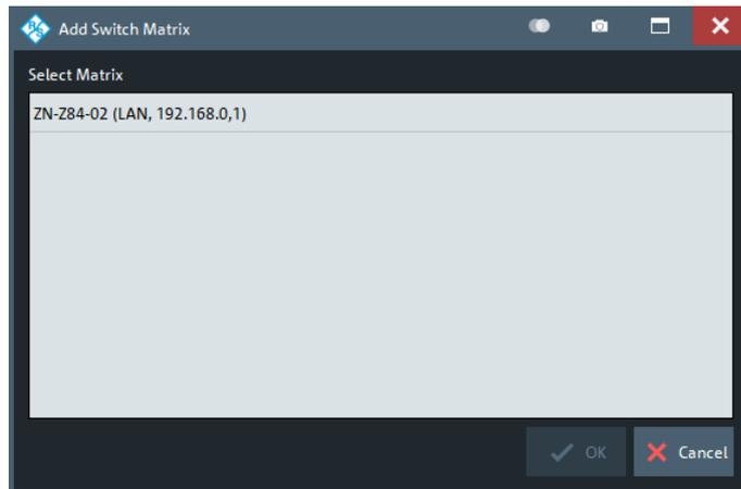
Select the required matrices and tap "OK" to add them to the RF connection configuration or tap "Cancel" to quit the dialog without adding a switch matrix to the RF connection configuration
