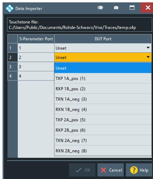
On the S-parameter board, the imported S-parameters are highlighted in the "Imported" color, which is blue by default (see ["Color Legend"](#) on page 781). E.g., if you map DUT ports 1 to 4 in the "Data Importer", then the background of the upper left 4x4 square on the S-parameter board is set to the "Imported" color:
