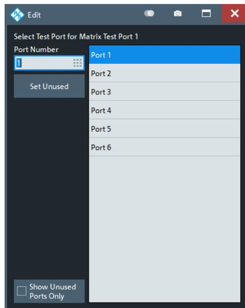
In the "Edit" dialog, define the appropriate test port or select "Set Unused" to delete the test port assignment. Configuration errors are displayed in balloon popups appearing at the lower left corner of the "Switch Matrix RF Connections" dialog.
