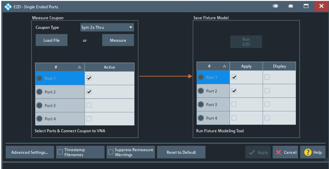
Figure 4-34: Fixture modeling: EZD – Single Ended Ports dialog
