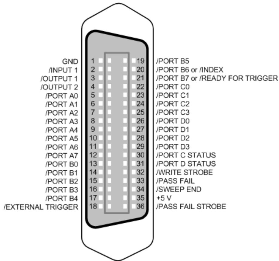
Figure 12-5: Pin assignment of the Universal Interface connector
