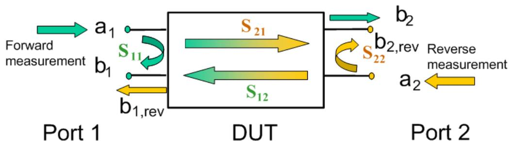
The predefined wave quantities can all be obtained with the same test setup, where a 2-port DUT is connected between the analyzer ports 1 and 2. The stimulus signal is provided by the analyzer port 1 or 2 ("Source Port").
