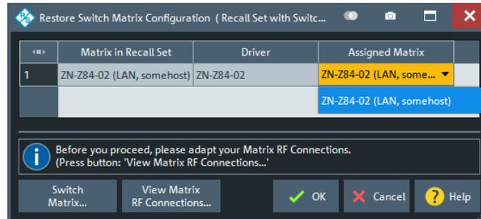
If no switch matrix of the same type exists, select "Switch Matrix" to open the [External Matrices dialog](#) that allows you to register/configure additional switch matrices.
