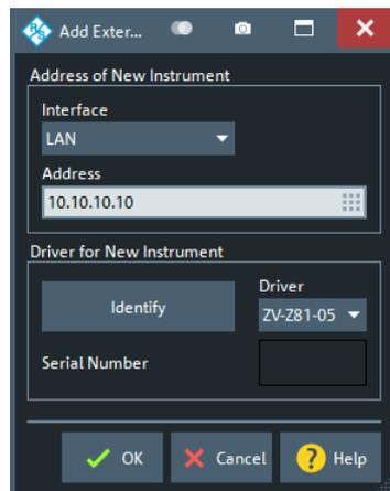
In the "Address of New Instrument" part, you can specify the required connection properties:
