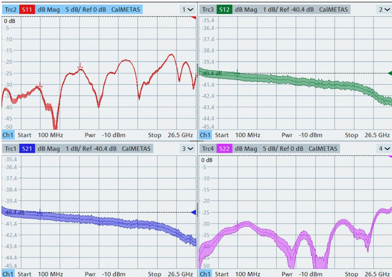
Figure 4-30: S-parameter measurements with uncertainty bands
