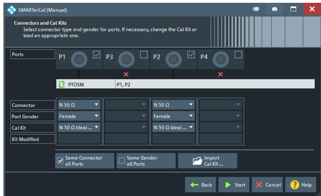
Figure 5-42: SMARTerCal(Manual), Step 2: Connectors and Cal Kits
