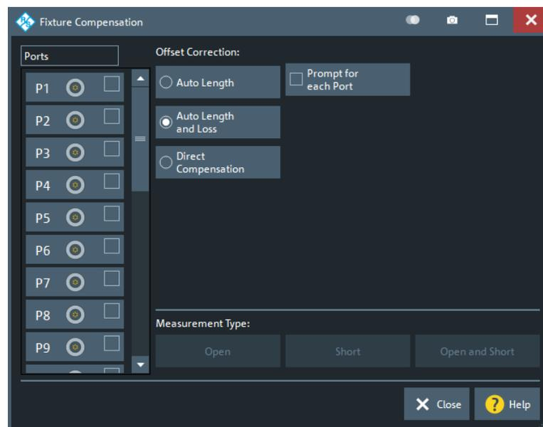
*Figure 5-61: Fixture Compensation dialog (for >4 ports)*
