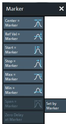
**Center = Marker / Start = Marker / Stop = Marker / Span = Marker**
