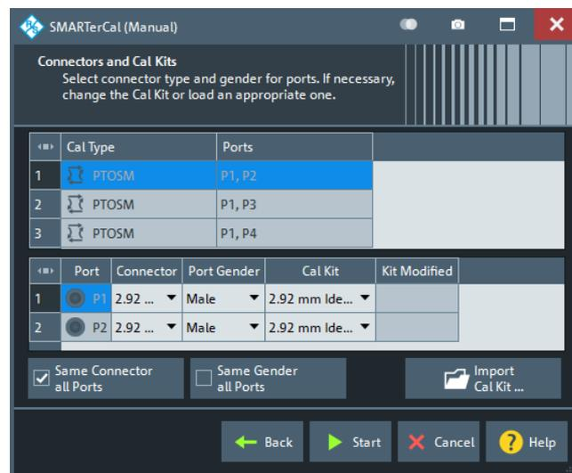
The upper part of the panel shows the previously configured SMARTerCal(s). Select the appropriate one to get access to the related port settings. For the individual calibrations, the functionality is the same as described for the single calibration version of the wizard (see ["Step 2: Connectors and Cal Kits"](#) on page 521).
