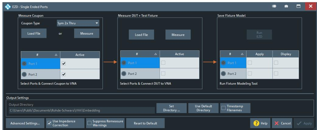
Figure 5-67: Fixture modeling dialog: EZD - Single Ended Ports
