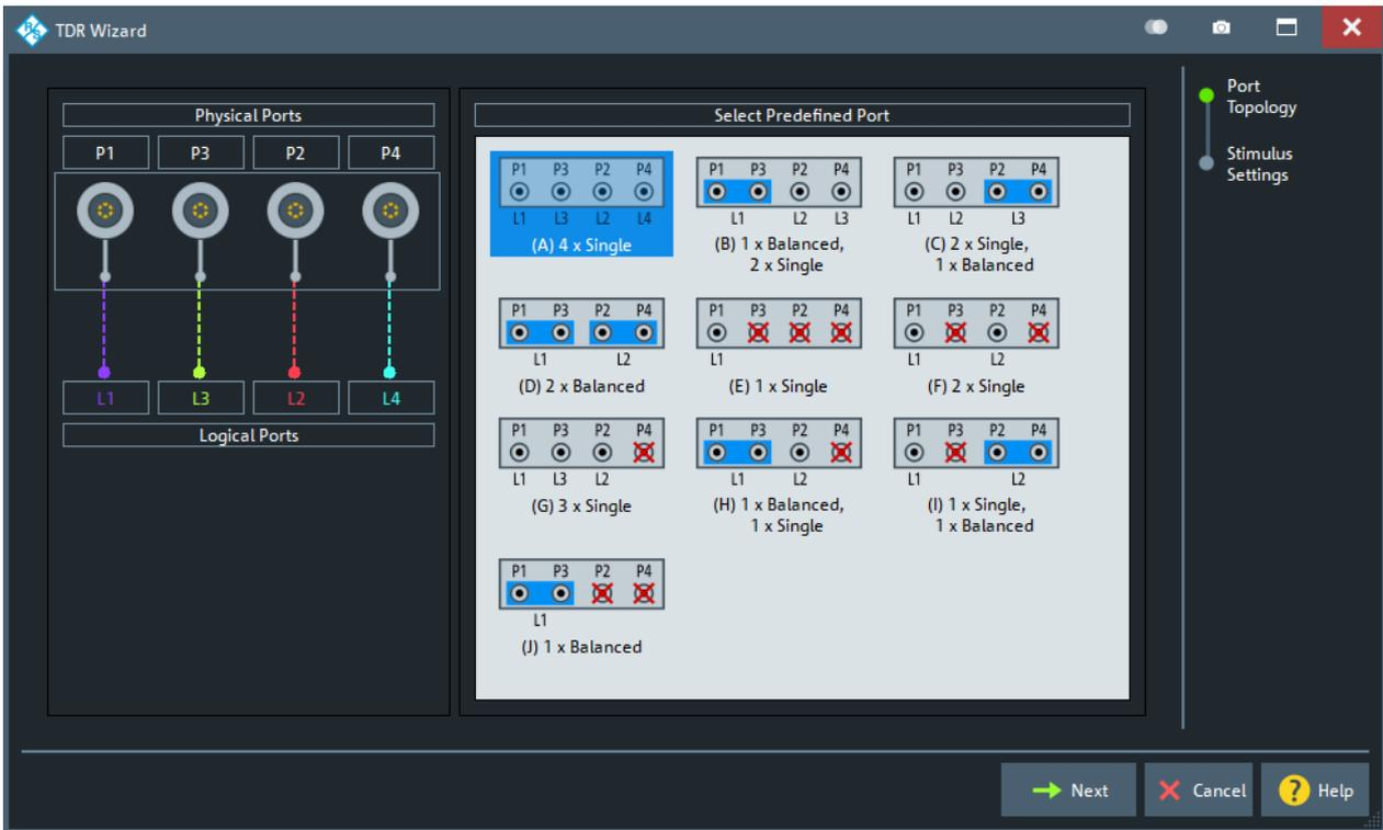
Figure 5-77: Port Topology step ( $\leq 4$  physical ports)
