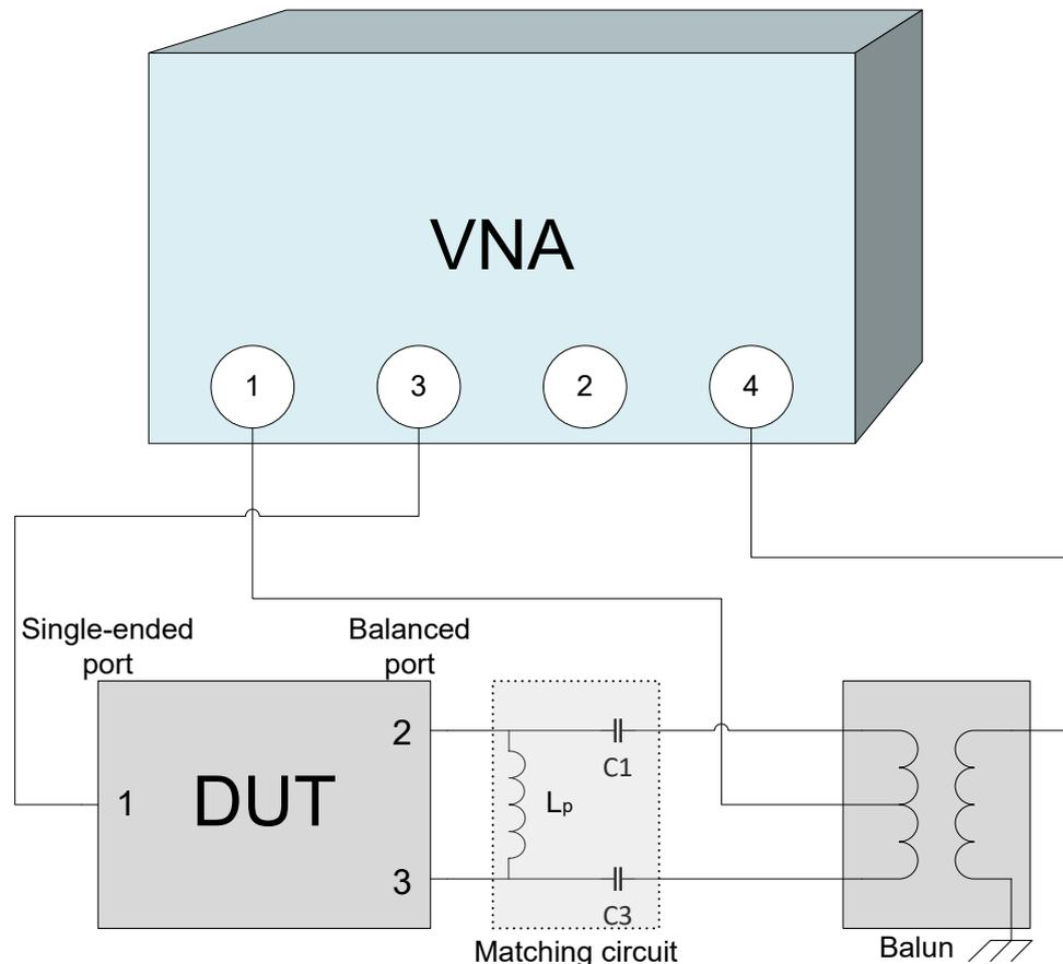
The idea of virtual embedding is to simulate the matching network and avoid using physical circuitry so that the analyzer ports can be directly connected to the input and output ports of the DUT. The matching circuit is taken into account numerically. The analyzer measures the DUT alone but provides the characteristics of the DUT, including the desired matching circuit.
