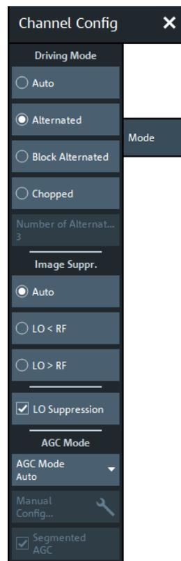
The controls on the "Mode" tab are organized in sections "Driving Mode", "Image Suppr." and "AGC Mode".
