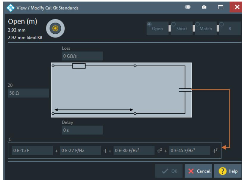
The diagram in the "View / Modify Cal Kit Standards" dialog depends on the standard type for which the dialog was opened. Moreover, it is possible to modify the circuit model using the buttons in the upper right of the dialog.
