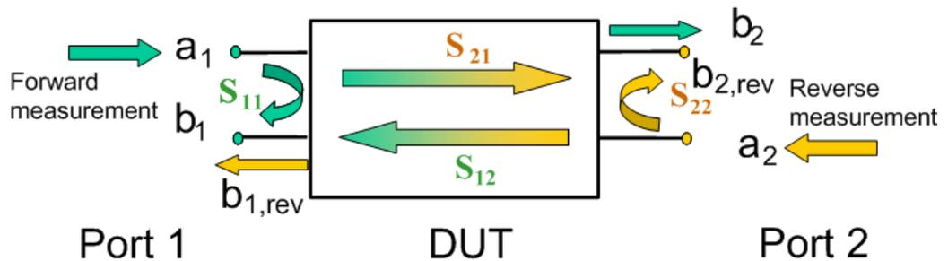
The figure above is sufficient for the definition of S-parameters but does not necessarily show the complete signal flow. In fact, if the source and load ports are not ideally matched, part of the transmitted waves are reflected off the receiver ports. An additional  $a_2$  contribution occurs in forward measurements, and an  $a_1$  contribution occurs in reverse measurements. The 7-term calibration types Txx take these additional contributions into account.
