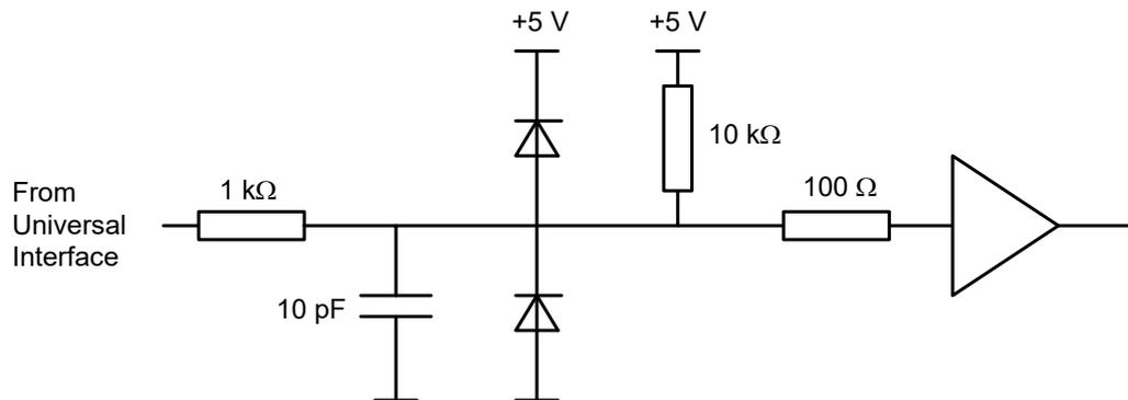
Figure 12-6: Circuit diagram of the input path
