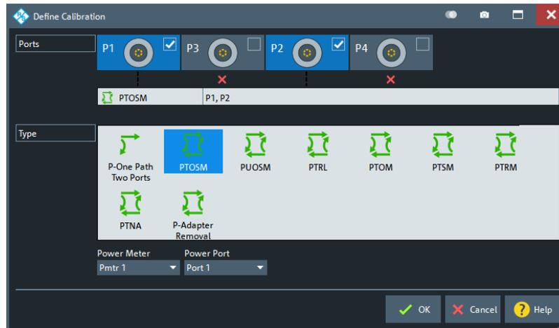
Figure 5-45: Define Calibration dialog (SMARTerCal)
