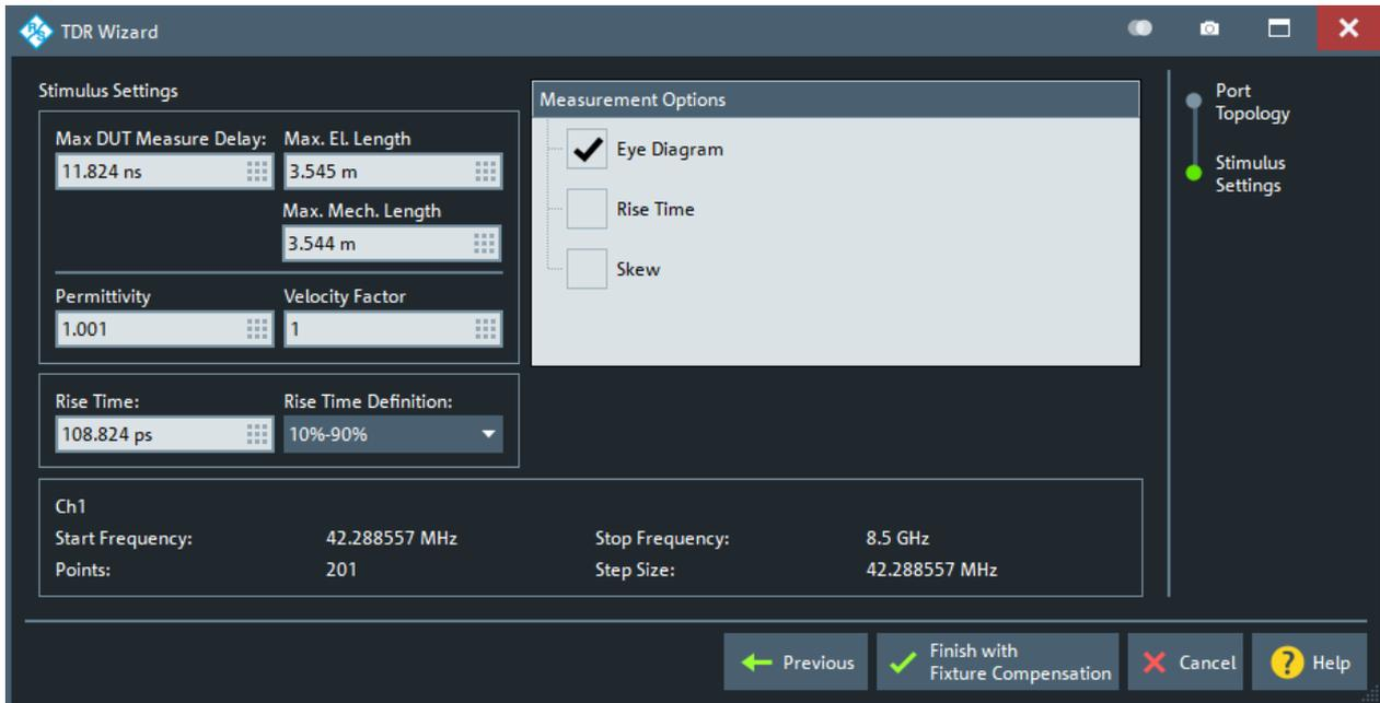
Once you have selected a measurement, you can finish the wizard and proceed to the [Fixture Compensation dialog](#) using the "Finish with Fixture Compensation" button.
