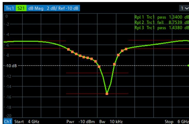
The limit line rules for logarithmic sweeps and segmented frequency sweeps with point-based x-axis also apply to ripple limit lines (see [Chapter 4.4.1.1, "Rules for limit line definition"](#), on page 147).
