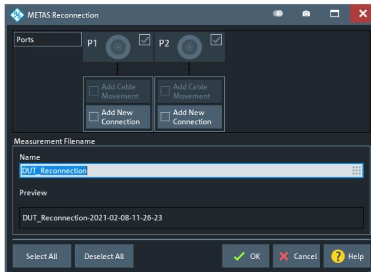
Both reconnections and cable movements contribute to the overall measurement uncertainty. In the METAS VNA Tools project created during the [METAS calibration](#), these events are registered in the so-called measurement journal. In addition, the results measured immediately after the event report are persisted in the project.
