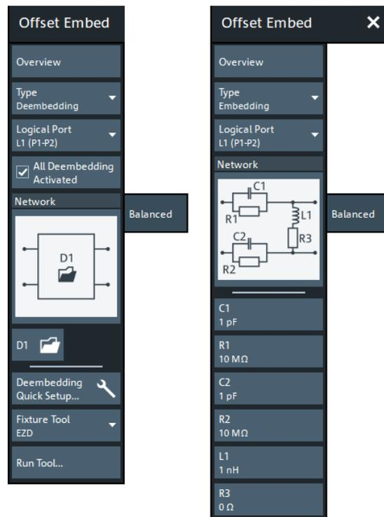
**Figure 5-71: Offset Embed > Balanced softtool**
