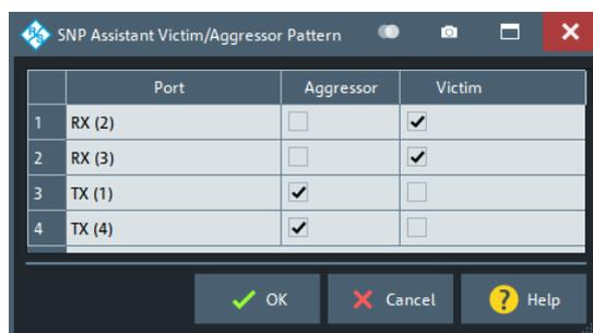
The V/A pattern above represents the crosstalk intention "As specified by topology wiring".
