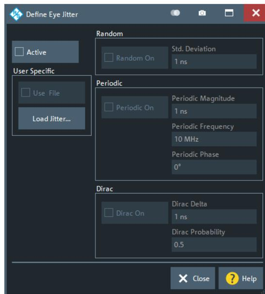
Four types of jitter can be configured and selectively enabled: random, periodic, Dirac and user defined. If enabled, the jitter is added at the start of each symbol period, and its magnitude depends on the parameters specified in the dialog.
