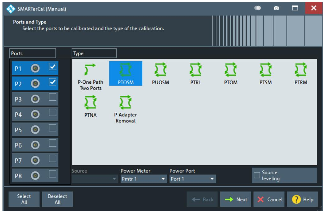
Figure 5-41: SMARTerCal(Manual), Step 1: Ports and Type (>4 ports)
