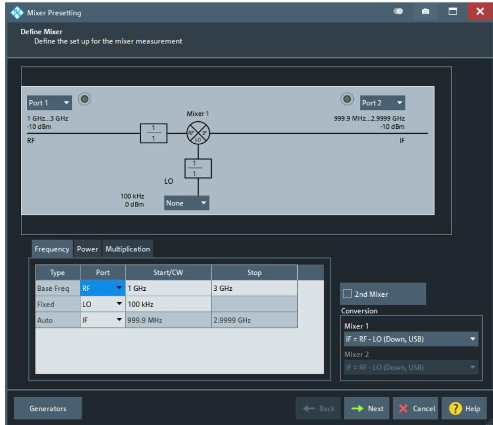
2. Select the mixer parameters to be measured. Depending on your selection, the required channels and traces are set up automatically; the active channel and its first trace will be renamed, all other channels and traces in the active recall set will be deleted.
