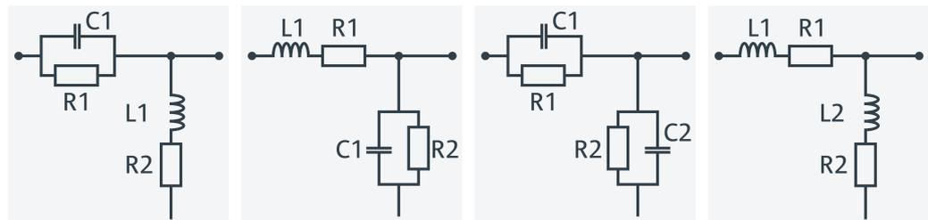
The following networks are composed of a shunt C or L (as seen from the analyzer port), followed by a serial C or L. They are named Shunt C, Serial L / Shunt L, Serial C / Shunt C, Serial C / Shunt L, Serial L.
