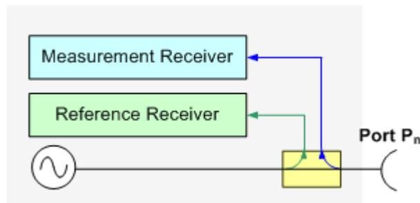
A measurement receiver calibration generally improves the accuracy of power (wave quantity) measurements. The correction data acquired in a frequency or power sweep is re-used if a "Time" or "CW Mode" sweep is activated.
