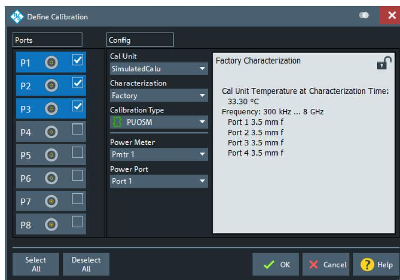
Figure 5-37: Define Calibration dialog (MultiCal, > 4 test ports)
