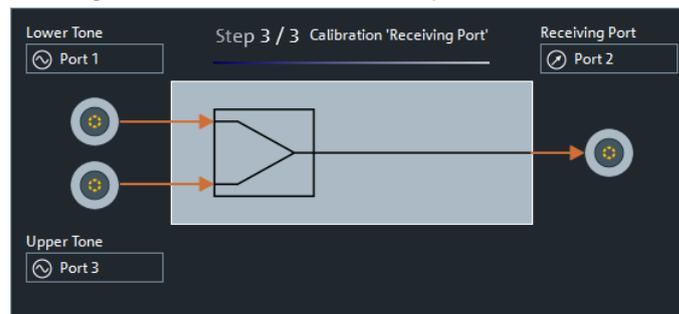
If a frequency conversion measurement is active, a second receiver power calibration is performed at the converted lower tone frequency.
