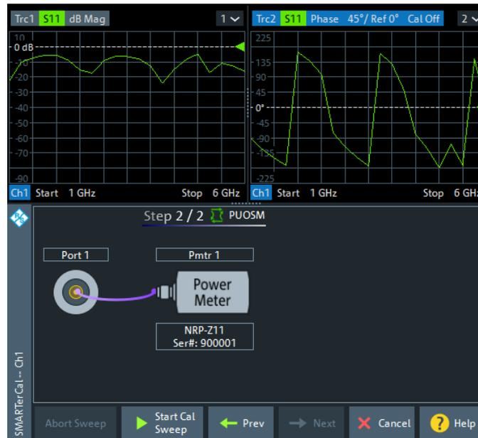
Use "Next"/"Prev" to navigate between the calibration substeps.
