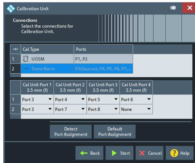
Figure 5-23: Multiple calibrations (and multiple port assignments)
