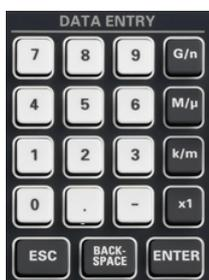
The keys in the DATA ENTRY keypad are used to enter numbers, units, and characters. The data entry keys are only enabled while the cursor is placed on a data input field in a dialog or in the Help navigation pane.
