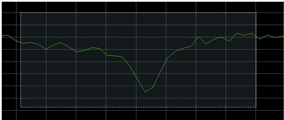
The zoomed view shows the selected rectangle, scaled in both horizontal and vertical direction. In general, the zoom window covers only a part of the sweep range; the horizontal distance between the sweep points increases. The reduced display range is indicated in an additional zoom line in the channel info area.
