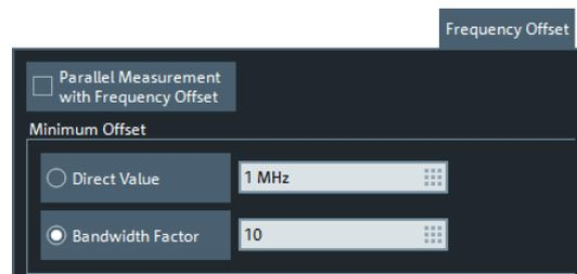
To get access to the "Frequency Offset" configuration, create multiple DUTs (on the R&S ZNB, set "Parallel Measurement" to "Enabled") and activate the "Frequency Offset" tab.
