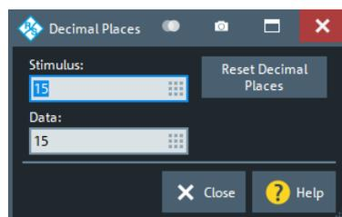
The allowed range is 1 (minimum precision) to 15 (maximum precision). "Reset Decimal Places" resets these numbers to their respective defaults, which is 15 in both cases.
