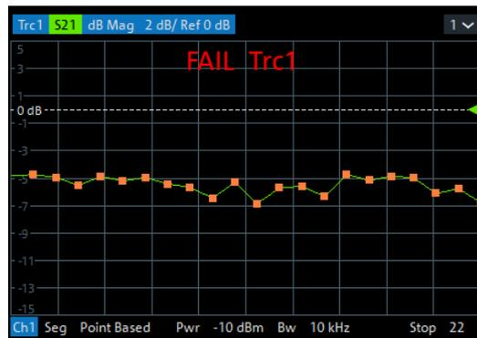
**Tip:** Overlapping limit line and ripple limit line segments are not displayed when a point-based x-axis is active; see [Chapter 4.4.1.1, "Rules for limit line definition"](#), on page 147.
