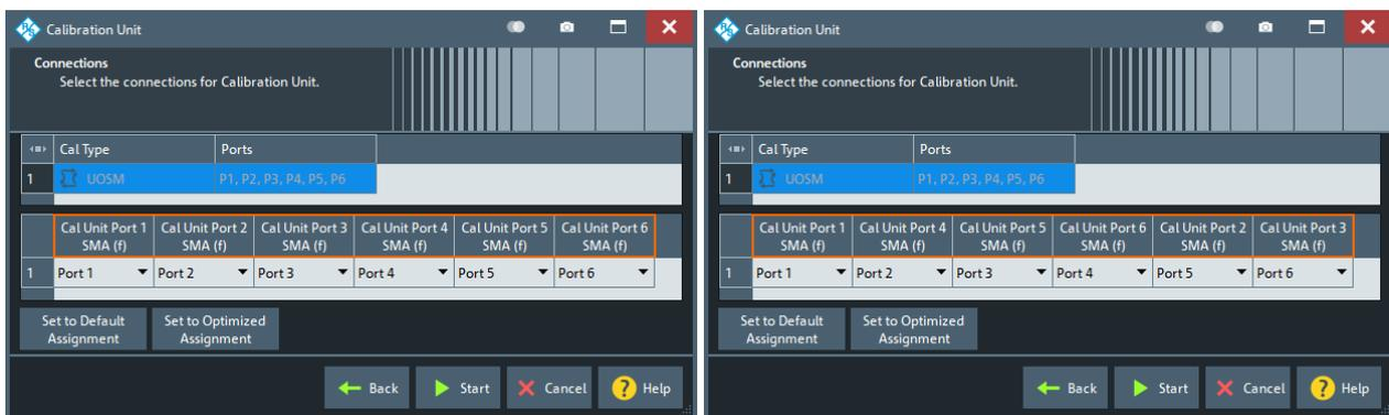
Figure 4-43: Optimized port assignment for 6-port R&S ZN-Z154
