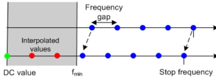
If the start frequency of the sweep is close to  $f_{\min}$ , then the sweep points can have to be shifted towards higher frequencies. If the last sweep point of the calculated harmonic grid exceeds the maximum frequency of the analyzer, then an error message is displayed, and another harmonic grid algorithm must be used.
