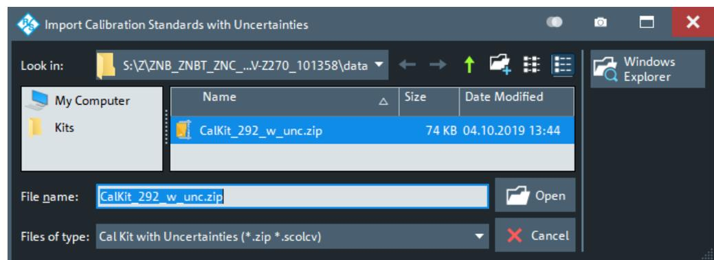
The imported cal kit is assigned to the selected [Connector](#) type; the name of the ZIP file is used as the cal kit name.
