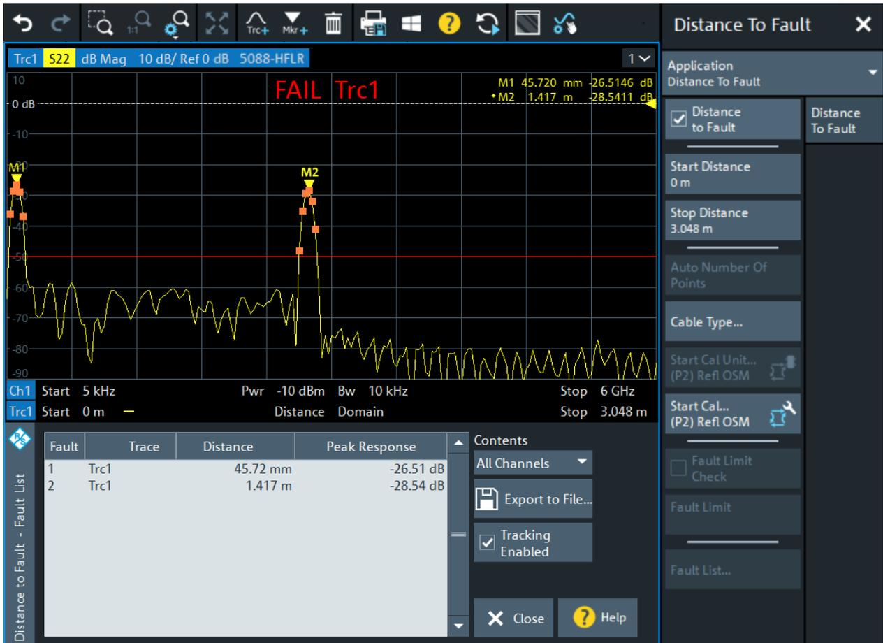
Adjust the frequency sweep to the length of the transmission line and the expected distance to fault:
