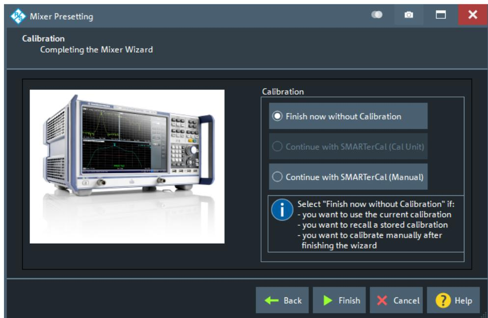
Depending on your selection, the wizard either closes without calibration or launches one of the mixer measurement-specific SMARTerCal wizards (see [Chapter 5.12.6.4, "SMARTerCal \(Cal Unit\) wizard for mixer mode"](#), on page 626 and [Chapter 5.12.6.5, "SMARTerCal \(Manual\) wizard for mixer mode"](#), on page 627).
