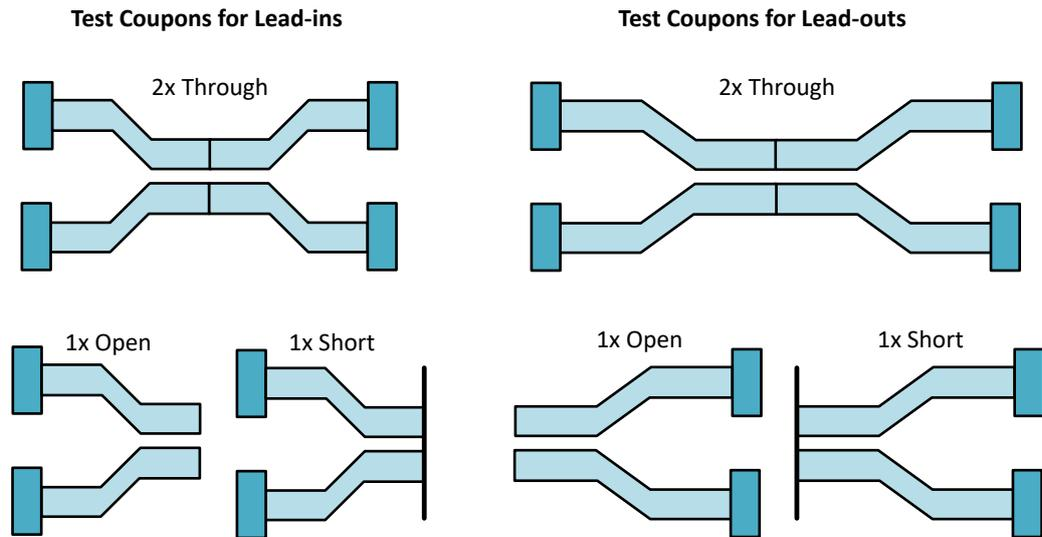
Figure 4-15: Test Coupons (balanced)
