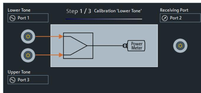
If a frequency conversion measurement is active, a second source power calibration is performed at the converted lower tone frequency (receiver frequency). This second source power calibration is the basis for the receiver calibration in step 3.
