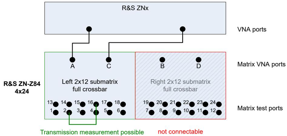
Figure 4-37: Unconnected right submatrix
