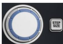
The rotary knob increases and decreases numerical values, scrolls within lists, activates controls and confirms entries. Turning or pressing the rotary knob is equivalent to the action of the "Cursor Up" and "Cursor Down" navigation keys or of the ENTER key in the DATA ENTRY keypad, respectively.
