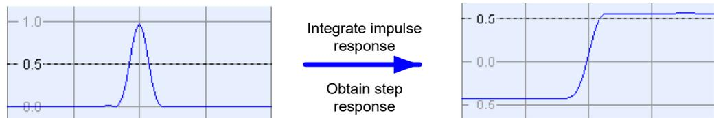
The step response is recommended for impedance measurements and for the analysis of discontinuities (especially inductive and capacitive discontinuities). The impulse response has an unambiguous magnitude and is therefore recommended for most other applications.
