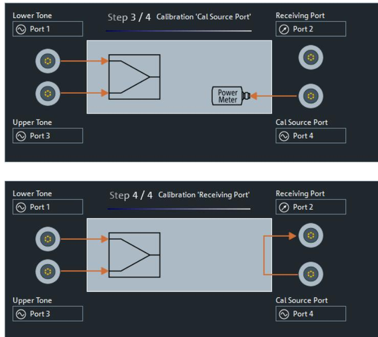
The progress of the calibration is monitored in the calibration sweep diagram, in close analogy to an ordinary power sweep; see ["Calibration Sweep Diagram"](#) on page 496.
