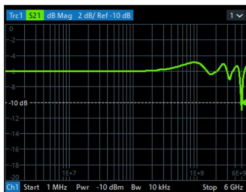
**Tip:** In "Log Freq" representation, limit lines and ripple limit lines appear as exponential curves; see [Chapter 4.4.1.1, "Rules for limit line definition"](#), on page 147.
