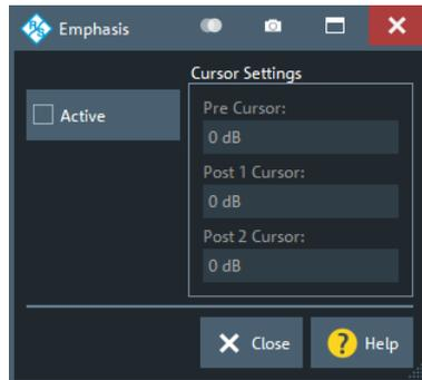
In transmission systems known losses of the channel are typically compensated already in the transmitter. The most common setting is to boost high frequencies compared to low frequencies since the channels show typically larger losses for high frequencies.
