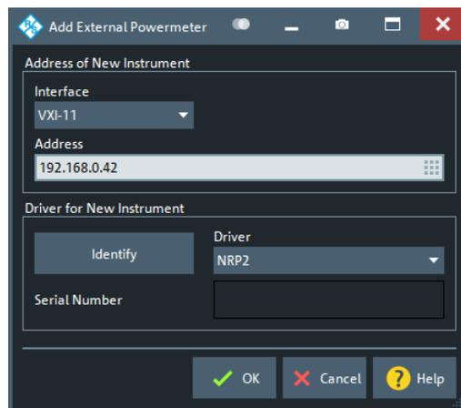
In the "Add External Power Meter" dialog, you can specify the instrument and connection properties:
