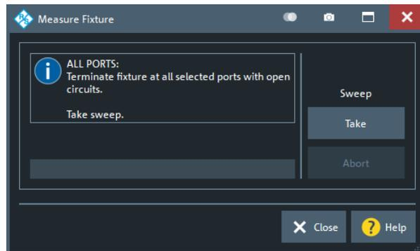
**Figure 5-62: Measure Fixture dialog: Auto Length (and Loss)**
