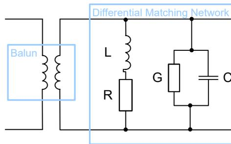
In contrast to standard balanced embedding (4-port), the matching circuit is only applied to the differential mode port (2-port). It can be specified via a Touchstone s2p file or by parametrizing a lumped "Shunt L, Shunt C" element model.
