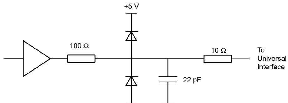
Figure 12-7: Circuit diagram of the output path
