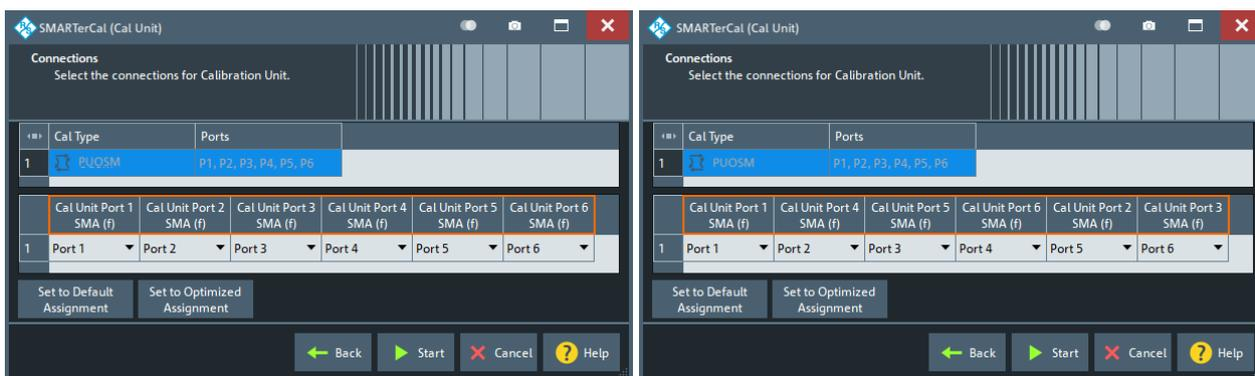
Figure 5-35: Optimized port assignment for 6-port R&S ZN-Z154
