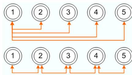
[For the mathematically inclined: the graph constructed from the calibration ports as nodes and the measured Throughs as edges must be connected.]
