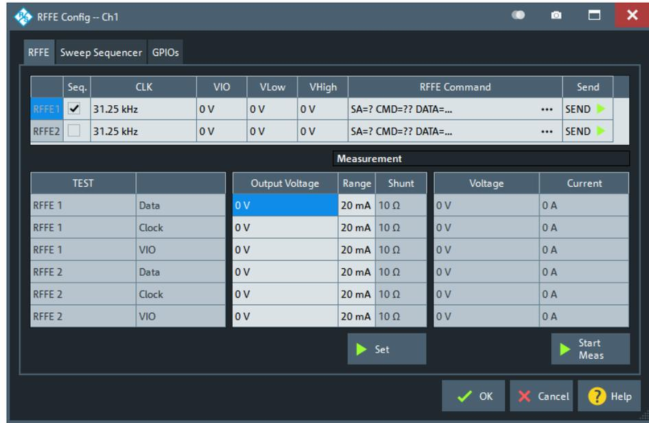
If the instrument is equipped with **variant 02** of the extension board, a slightly different user interface is shown. The "Measurement" columns are hidden and the remaining content of the RFFE and GPIO tab are presented on a single "Control" tab.
