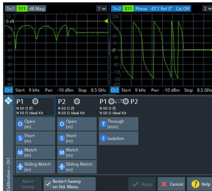
The analyzer performs a calibration sweep for the measured quantity  $S_{21}$ . The magnitude and phase of the result is displayed in two diagrams, together with the expected typical result for a Through standard. The similarity of real and expected traces indicates that the Through standard has been properly connected. After the R&S ZNB/ZNBT has completed the calibration sweep and calculated the correction data, the "Apply" button is enabled.
