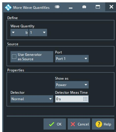
The notation for wave quantities follows the usual scheme of the vector network analyzer:
