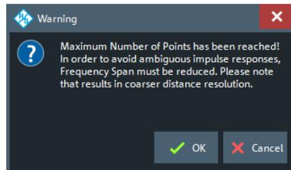
"OK" reduces the frequency span to  $\Delta f = v \cdot c_0 \cdot N_{max} / (2.6 \cdot d_{stop})$ , which makes  $N_{max}$  sweep points sufficient for unambiguous display (see the formula above). However, this reduction of the frequency span comes at the cost of coarser distance resolution.
