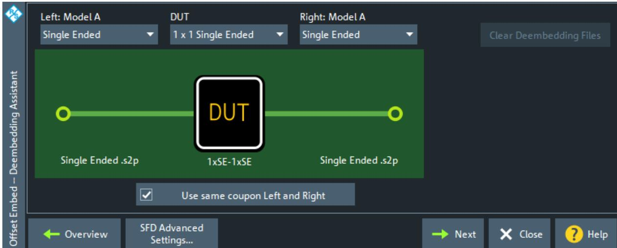
Depending on the selected [fixture tool](#), it narrows down the selectable [DUT](#) types and [test coupon models](#).
