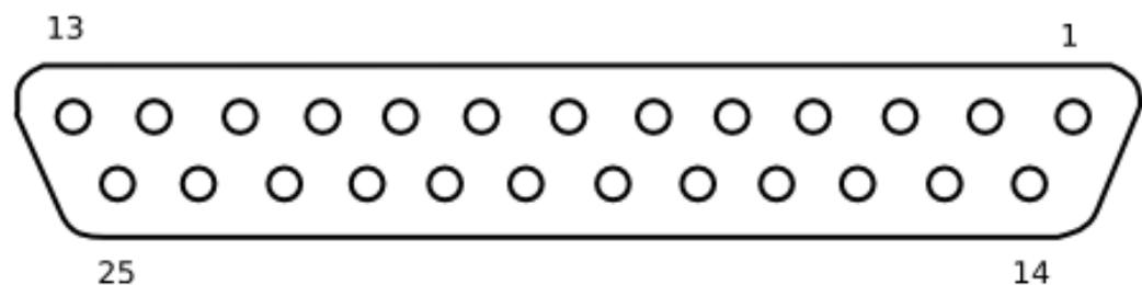
Figure 12-9: D-sub 25-pin female connector, front view
