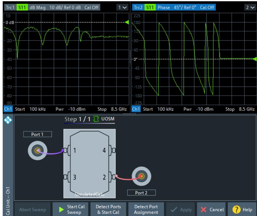
In the upper part of the "Cal Unit" screen, the R&S ZNB/ZNBT shows the calibration sweep diagrams for the currently measured S-parameter. The lower part visualizes the active port assignment and the measurement progress.
