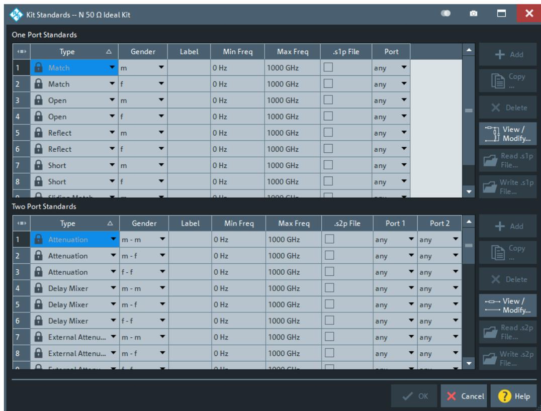
One port and two port standards are listed in two separate tables. Most of the buttons on the right side are available only if the "Kit Standards" dialog was opened for a user-defined calibration kit.
