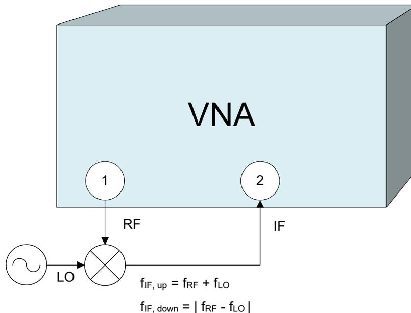
In this example, the transmission parameter  $S_{21}$  corresponds to the mixer's conversion gain.
