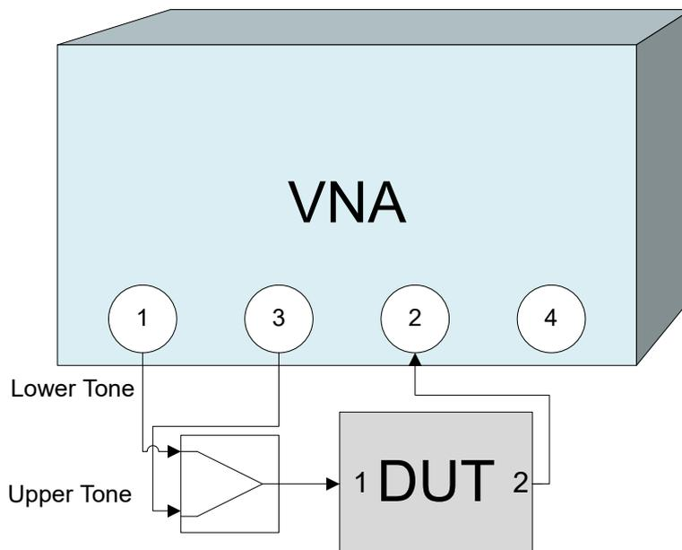
For a R&S ZNBT with more than 8 ports the lower and upper tone could be provided by ports 1 and 9, for example.
