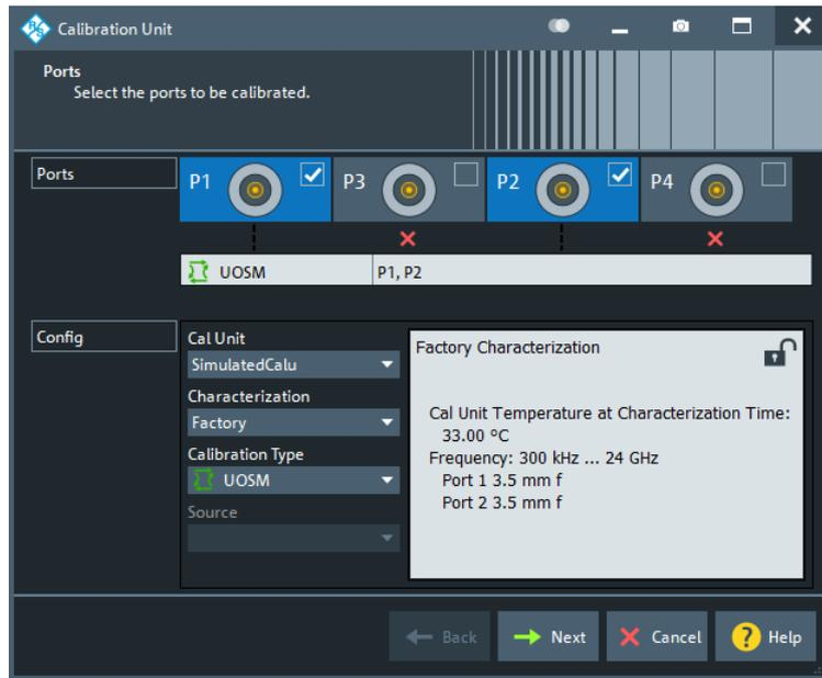
Figure 5-12: Calibration Unit wizard, step 1: Ports
