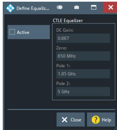
Similar to the usage of emphasis the equalization targets to improve the signal quality at the receiver end of the transmission system. The building block "Equalize" simulates a continuous-time linear equalizer (CTLE) which is typically realized as an analog circuit in receivers.
