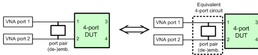
The two port pair (de-)embedding networks in the figure below are based on port pairs 1, 2 and 1, 3 with appropriate sets of 4-port S-parameters.
