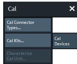
The buttons in the "Cal Devices" tab open the following dialogs:
