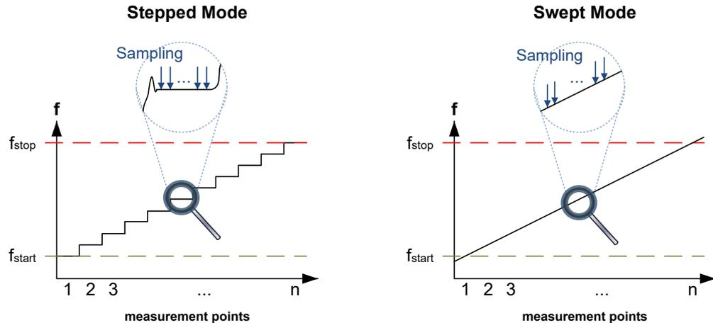
Apart from the loss in precision, there can be other technical reasons that prevent the swept mode from being advantageous. For instance if the sweep is triggered by events caused by external devices such as part handlers, generators or power meters, the sweep (implemented in hardware) has to be interrupted by the software regularly and cannot proceed autonomously after the initial phase lock.
