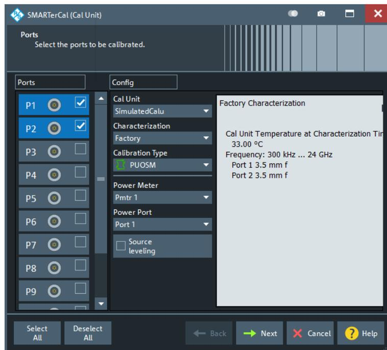
Figure 5-32: SMARTerCal (Cal Unit), Step 1: Ports (> 4 Ports)
