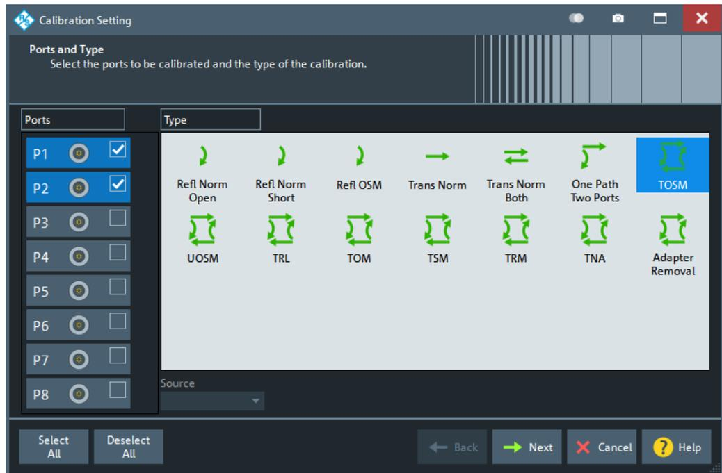
Figure 5-24: Calibration Presetting: Ports and Type (> 4 test ports)
