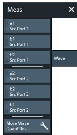
The "More Wave Quantities..." button opens the [More Wave Quantities](#) dialog which allows to select an arbitrary [wave quantity](#), e.g. for different source ports or higher port numbers.
