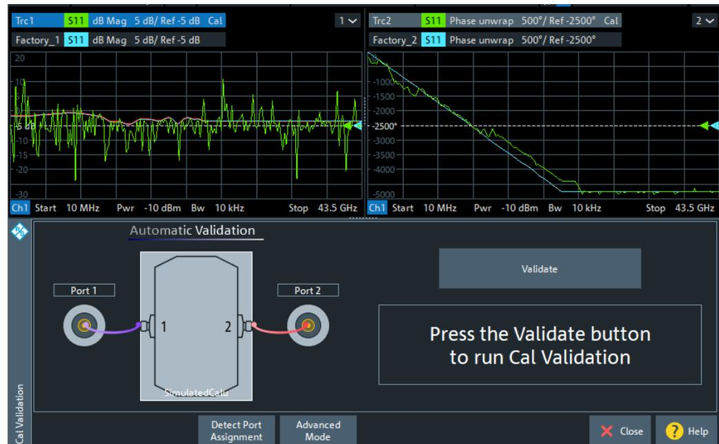
The validation logic proceeds through the connected ports  $p \in \{1, \dots, 4\}$  in ascending order, measuring  $S_{pp}$  for the Open, Short and Match standard. It then compares the measured  $S_{pp}$  values with the corresponding reflection S parameters of the cal unit's factory characterization. The on-screen feedback indicates success ("PASS"), failure ("FAIL") or provides a warning about undetected ports.
