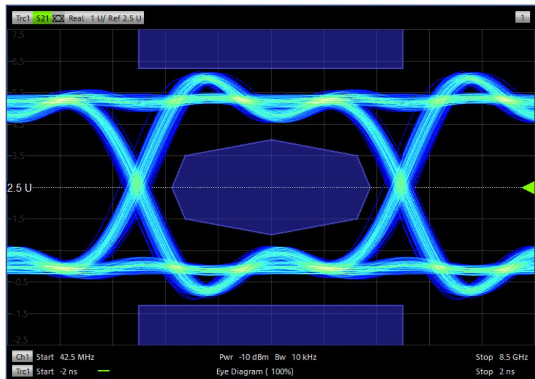
Figure 4-18: Eye diagram (NRZ modulated)
