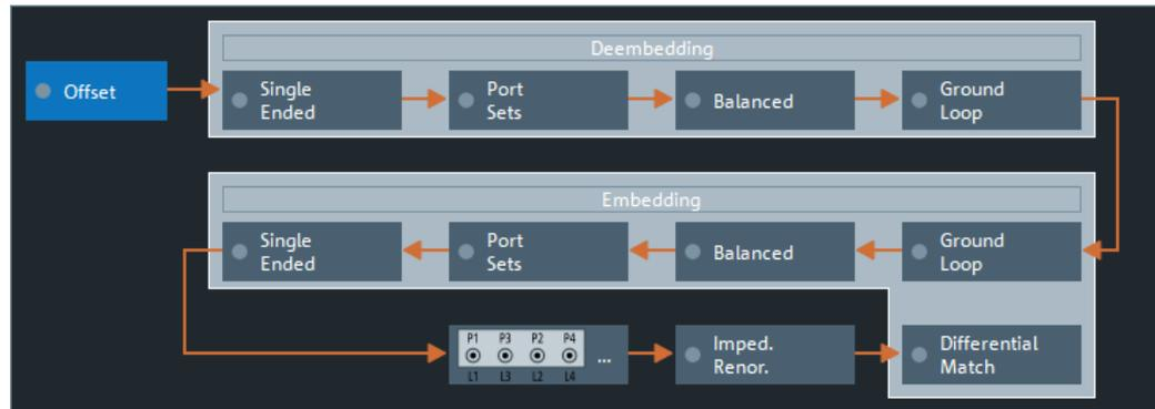
Figure 5-59: Offset Embed dock widget: Overview (Calculation Flow)
