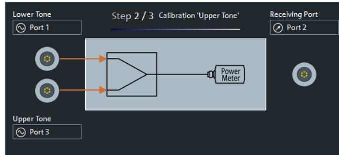
For frequency conversion measurements, no new source power calibration at the receiver frequency is performed.
