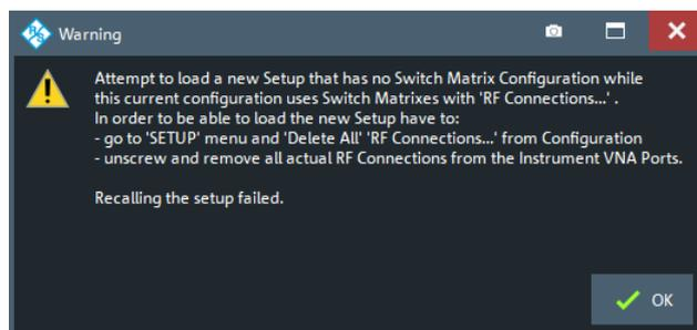
If the recall set to be loaded contains a switch matrix configuration and no differences to the current switch matrix configuration are detected, the recall set is loaded without further inquiry. Otherwise you are asked if you want to adapt the configuration:
