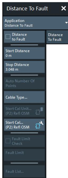
A standard DtF measurement is prepared in the order from top to bottom:
