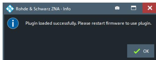
The firmware must be run as administrator to add or remove custom plugins. Once installed, standard user privileges are sufficient to use a plugin's functionality.
