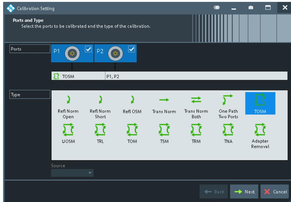
**Tip:** For a R&S ZNBT with more than 4 ports, the graphical port representation is replaced by a generic port list. The selection logic is unchanged.
