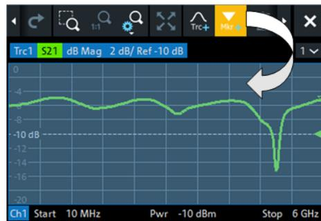
The marker appears on the target diagram's active trace. The marker info field displays the stimulus value (x-axis value) and response value (y-axis value) at the marker position. The response value varies as the analyzer continues performing sweeps.
