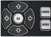
The keys in the NAVIGATION keypad are used to navigate within the touchscreen and the help system, to access and control active elements.
