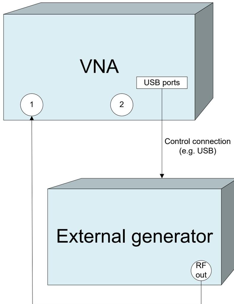
External generators must be configured in the System – [Setup] softtool before they are available as additional sources. Configured generators appear in many control elements of the R&S ZNB/ZNBT, e.g. in the "More Ratios", "More Wave Quantities", port configuration and power calibration dialogs.
