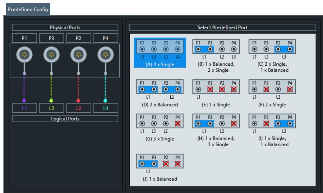
The port configurations are arranged in the list to the right. The resulting port assignment is shown on the left-hand side of the "Predefined Config" tab.
