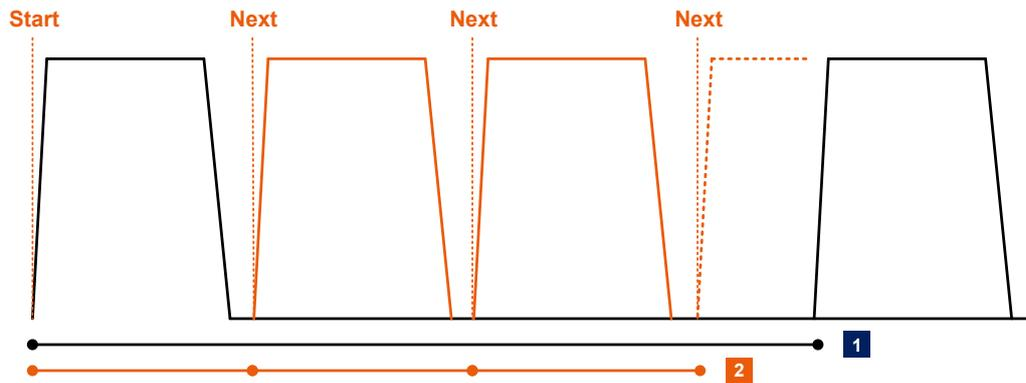
**Figure 4-28: Configured vs. effective pulse period (high-low, synchronized)**
