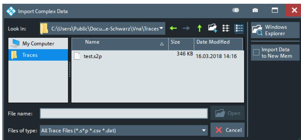
On loading data from a trace file with several traces, the analyzer displays a dialog to select one or more of the traces stored in the file (see [Chapter 5.5.11.3, "Select Parameter dialog"](#), on page 385). E.g., for an \*.s2p Touchstone file, the box offers all four 2-port S-parameters (see [Chapter 4.4.2.1, "Touchstone files"](#), on page 154).
