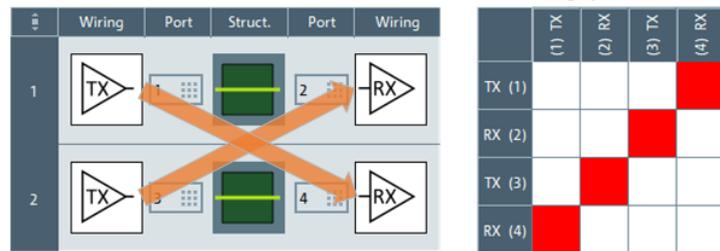
"NEXT (Near-End Crosstalk)" requires two DUT structures with inverse wiring (TX of structure 1 and RX of structure 2 on the same side of the DUT).
