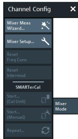
Most of the "Mixer Mode" buttons are only enabled if the mixer measurement is set up properly. They open wizards or dialogs:
