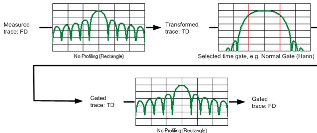
The shape, width and position of the time gate affect the gated frequency domain trace. The window type selection in the "Define Transform" dialog is ignored. The selected window is used again when the TD trace is displayed ("Time Domain: On").
