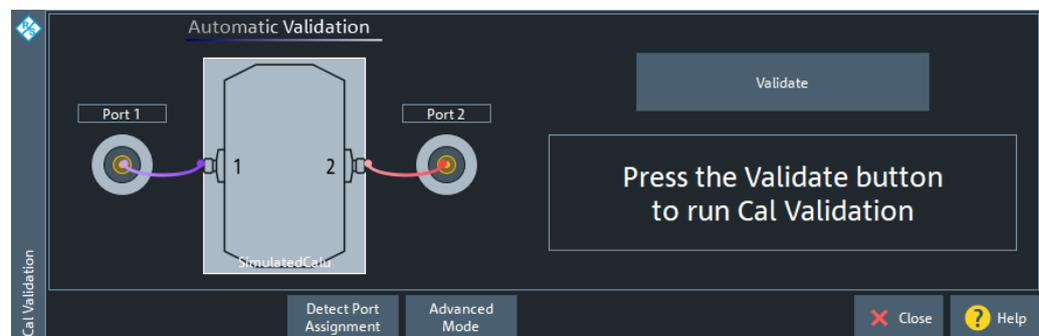
Use "Detect Port Assignment" to detect the current port assignment (after reconnecting the calibration unit).
