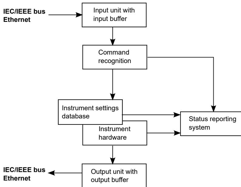
The individual components work independently and simultaneously. They communicate with each other with so-called messages.
