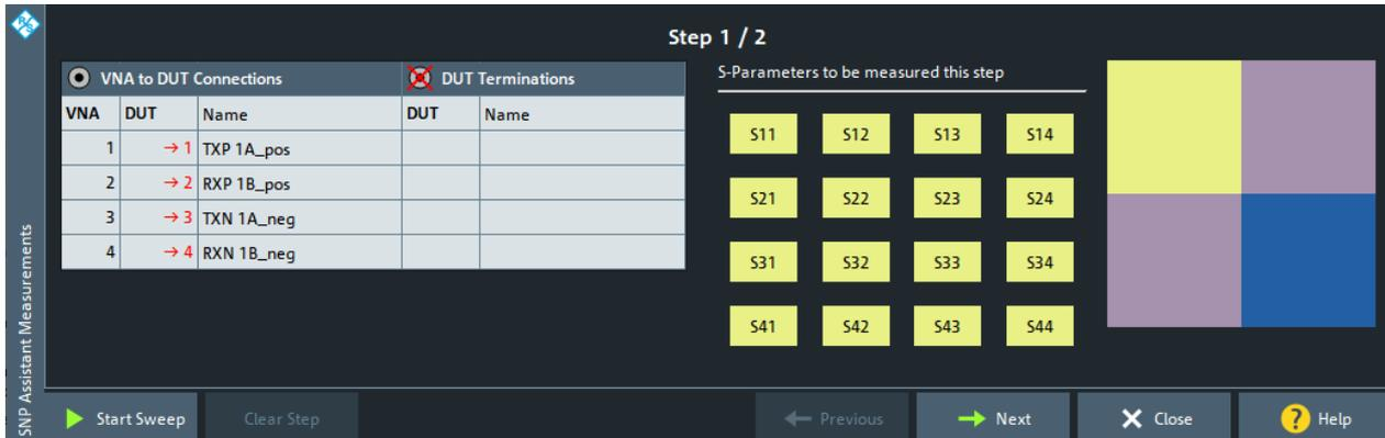
Depending on the number of ports on the VNA (and connected switch matrices), the number of DUT ports, and the S-parameters you do not assume "ideal", the SNPA algorithm determines the required measurement steps. The steps are optimized w.r.t. the number of cable changes.
