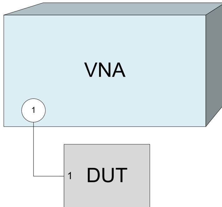
You can also use the basic transmission test setup, e.g. if you want to measure reflection and transmission parameters in parallel.
