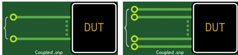
Figure 5-75:  $n > 1$  coupled input ports (single-ended | balanced)
