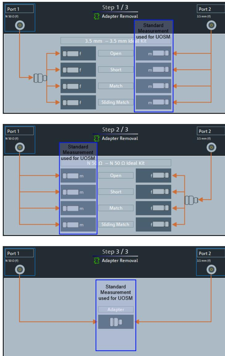
**Figure 4-9: Adapter Removal vs. UOSM**
