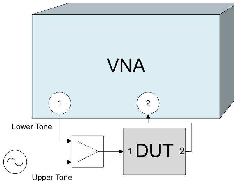
The lower tone signal is generated at port 1, the upper tone is provided by the external generator. Both signals are combined externally and fed to the DUT input. The intermodulation quantities can be measured at the DUT output (transmitted wave b2). It is possible to interchange the ports no. 1 and 2.
