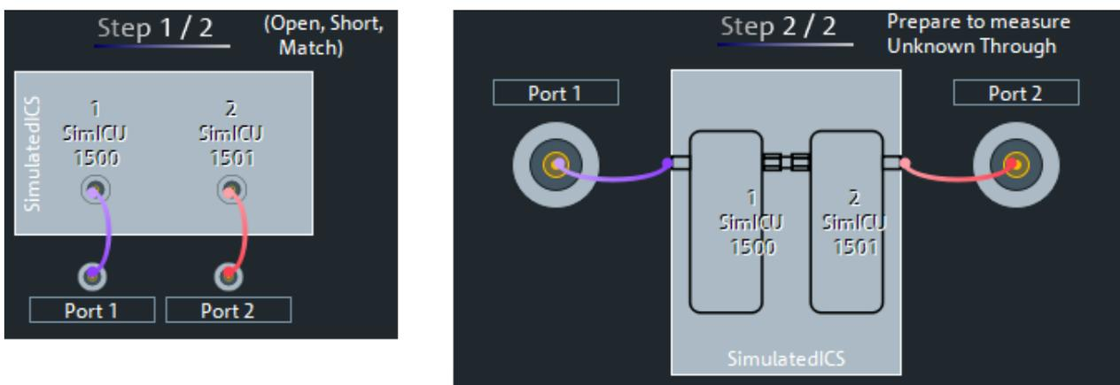
Figure 5-19: Automatic calibration: inline calibration system
