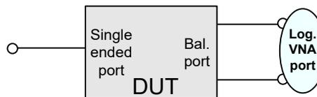
**4 physical ports:** Reflection and transmission measurements on 1 or 2 balanced ports**Single-ended (unbalanced) ports**
