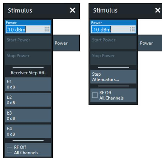
left = R&S ZNB with [Receiver step attenuators](#) and 4 physical ports
