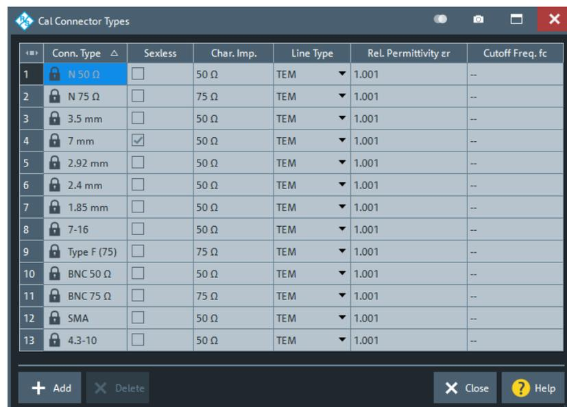
The list shows the available connector types with their name ("Conn. Type") and polarity ("Sexless"). The remaining columns in the list are described below.
