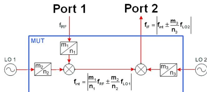
The figure above also shows the possible output frequencies of the two mixers. The actual values of  $f_{\text{int}}$  and  $f_{\text{IF}}$  depend on the RF and LO frequencies and of the measured conversion (lower sideband or upper sideband with up- or down-conversion). The analyzer automatically calculates all frequencies and sets its receiver according to the settings made.
