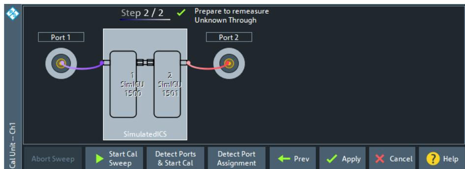
5. Connect the DUT to the calibrated setup and perform the required measurements.
