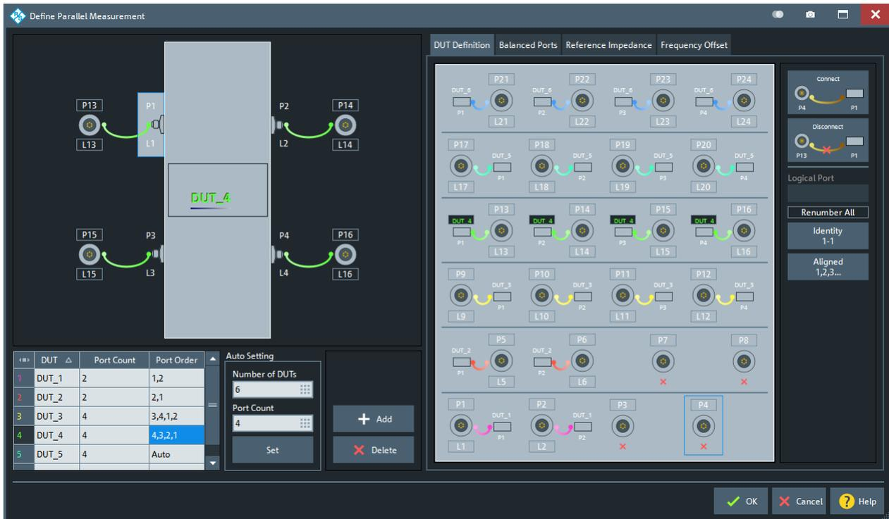
Figure 5-54: Define Parallel Measurement (R&S ZNBT with 24 ports)
