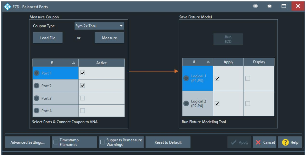
Figure 4-35: Fixture modeling: EZD – Balanced Ports dialog
