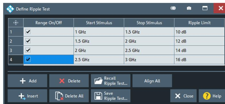
The "Define Ripple Test" dialog contains a table to edit the individual ranges of the ripple check ranges. The buttons below the table extend, shorten, or reorder the range list and save/recall ripple test data.
