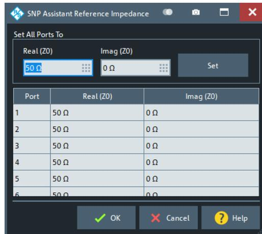
Use the controls in the "Set All Ports To" section to set a common reference impedance for all ports.
