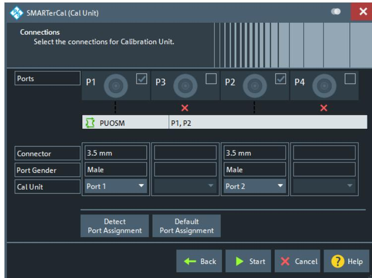
Figure 5-33: SMARTerCal (Cal Unit), Step 2: Connections (single)
