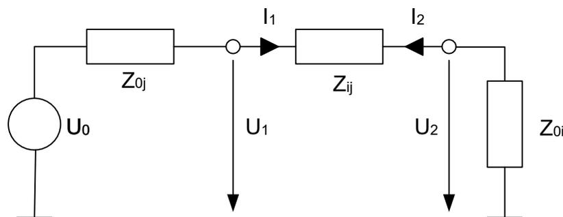
The calculation formula of a converted serial transmission impedance  $Z_{ij}$  depends on the waveguide circuit theory according to which [Reference impedances](#) are calculated.
