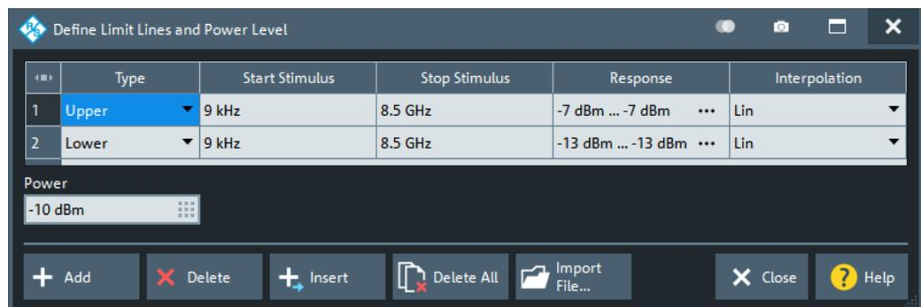
The available GUI elements for the limit line definition are the same as in the general-purpose limit line setup dialog. For their description, see [Chapter 5.6.1.2, "Define Limit Lines dialog"](#), on page 391.
