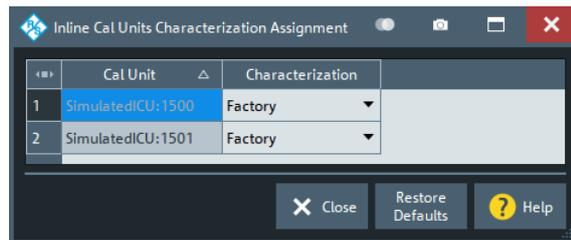
**Tip:** If the characterization wizard is password-protected, the "Characterization" button is unavailable. Use this functionality to prevent inadvertent activation of inappropriate characterizations. See ["Authentication"](#) on page 542.
