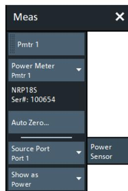
The standard test setup for a "Power Sensor" measurement involves one analyzer source port and a power sensor. The power sensor is connected to the VNA (e.g. to
