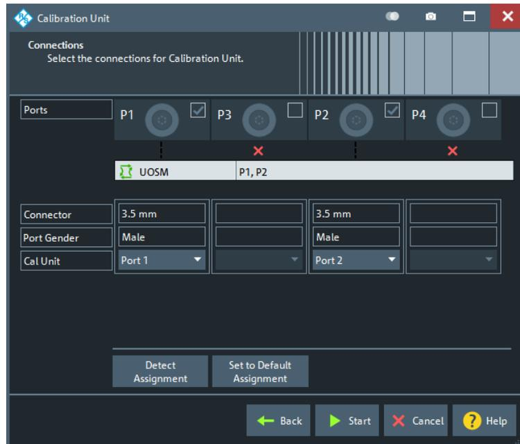
Figure 5-15: Calibration Unit wizard, step 2: Connections
