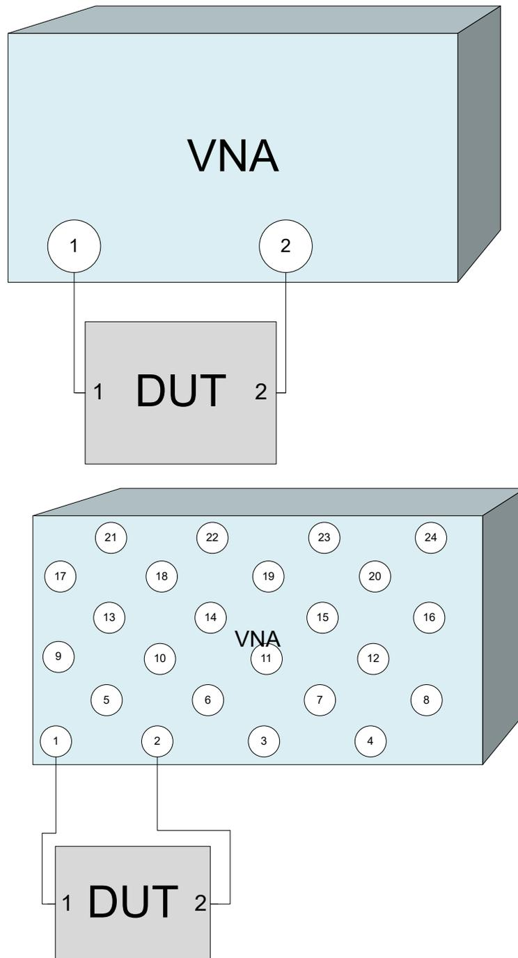
1. Connect the DUT between test ports 1 and 2 of the network analyzer as shown above.
