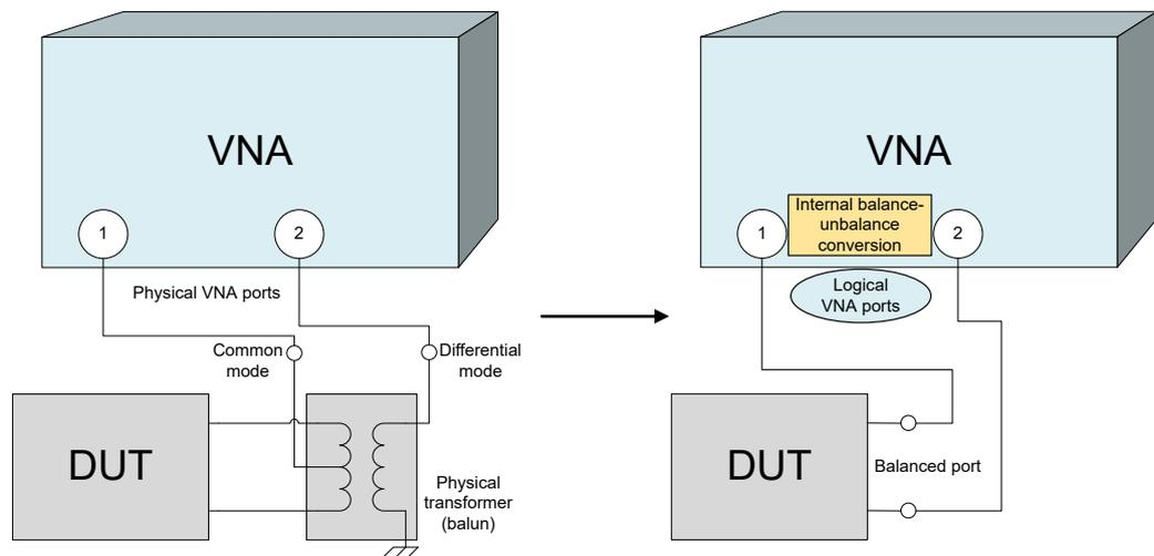
Unbalance-balance conversion avoids the disadvantages of real transformers:
