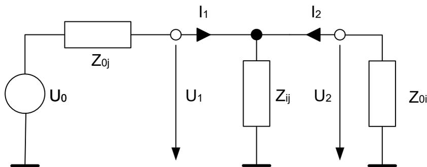
The calculation formula of a converted parallel transmission impedance  $Z_{ij}$  depends on the waveguide circuit theory according to which [Reference impedances](#) are calculated.
