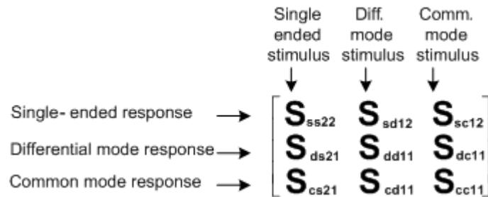
4. DUT with two balanced ports or one balanced and two single-ended ports. Both device types are fully characterized by 4x4 mixed mode S-matrices.
