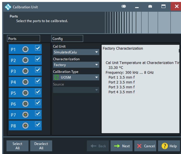
Figure 5-14: Calibration Unit wizard, step 1: Ports (> 4 test ports)
