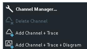
The settings in the context menus correspond to the most common functions in the Channel – [Channel Config] > "Channels" softtool tab, the "Stimulus" softtool (opened via Stimulus hardkeys), the Channel – [Sweep] > "Sweep Params" softtool tab, and the Channel – [Pwr Bw Avg] softtool.
