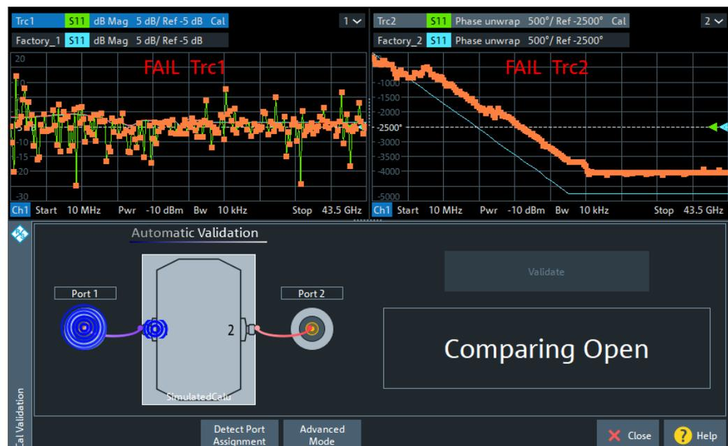
For a channel with more calibrated ports than cal unit ports available, you can change the port assignments and rerun the automated validation. Or you can switch to advanced mode and validate each port manually.
