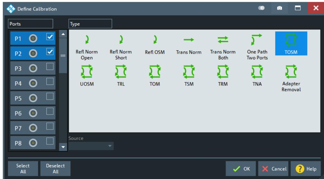
Figure 5-29: Define Calibration dialog (manual, > 4 test ports)
