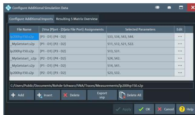
The source data files (first column), the mapping between physical ports and data file ports (second column), and the S-parameters to be overwritten (third column) can be defined during [Add/Insert](#). The text box below the table shows the full path to the data file of the selected row.
