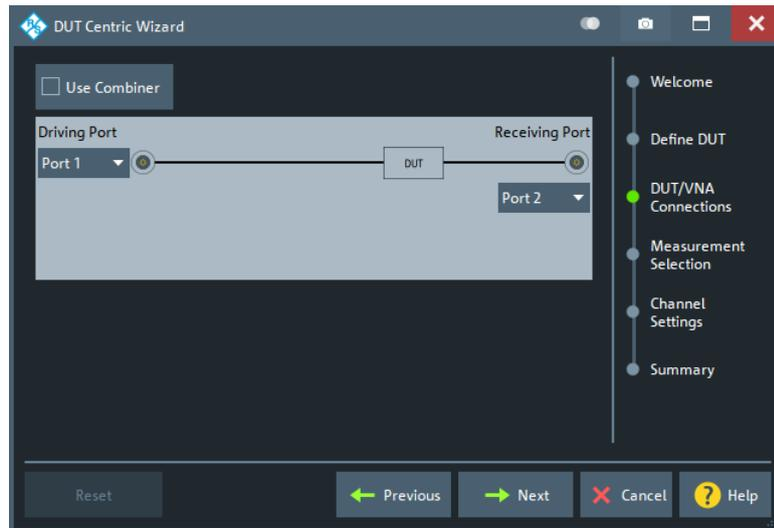
Figure 5-91: Amplifier/VNA connections
