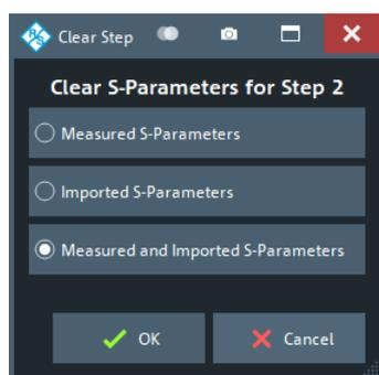
You can then either measure these S-parameters, or import their traces using the buttons in the step's [button grid](#).
