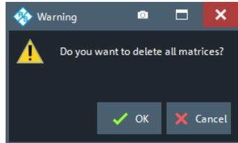
Either select "OK" to remove all switch matrices from the RF connection configuration, or "Cancel" to quit the dialog without removing a switch matrix.
