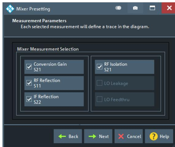
**Note** that LO parameters can only be measured if a VNA port was selected as the respective LO in the previous step. This in turn requires a second internal source (see [Chapter 4.7.16, "Second internal generator"](#), on page 265).
