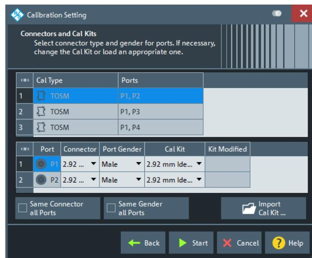
The upper part of the panel shows the previously configured calibrations. Select the appropriate one to get access to the related ports. For the individual calibrations, the
