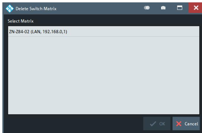
Select some matrices and tap "OK" to remove them from the RF connection configuration or tap "Cancel" to quit the dialog without removing a switch matrix from the RF connection configuration.
