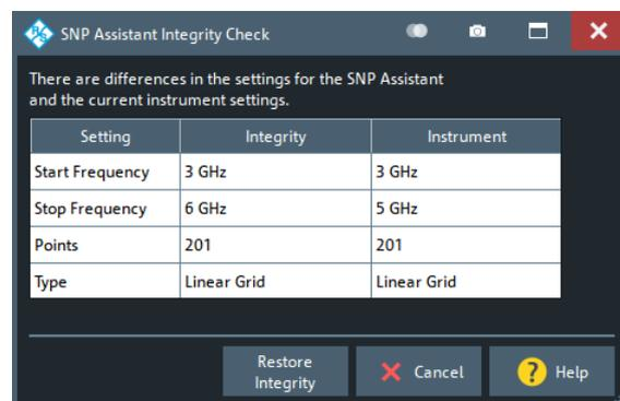
If the check fails, you can either adjust the channel's sweep settings to the project's sweep settings and continue with the measurement sweep ("Restore Integrity"), or "Cancel" the measurement sweep.
