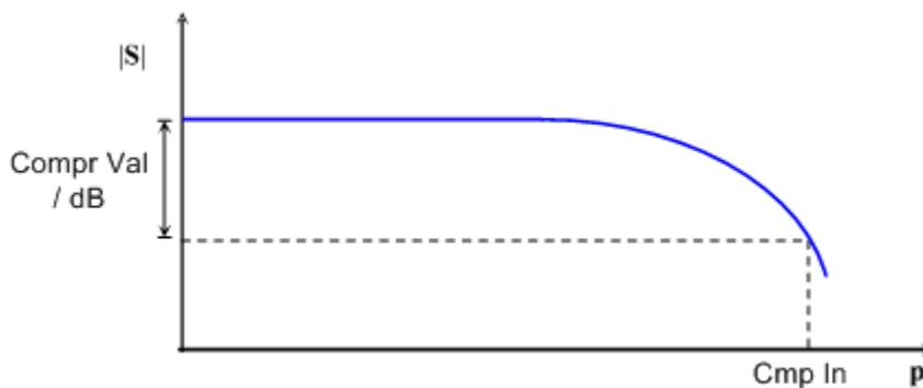
The compression point is a measure for the upper edge of the linearity range of a DUT. It is close to the highest input signal level for which the DUT shows a linear response, so that the magnitude of all S-parameters remains constant).
