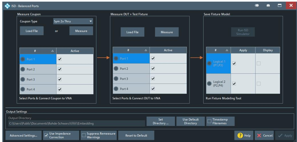
Figure 5-66: Fixture modeling dialog: ISD - Balanced Ports
