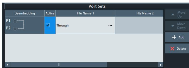
The "Port Sets" panel can also be activated by selecting the [Port Sets tab](#). Refer to its description for background information, parameters and additional remote commands.
