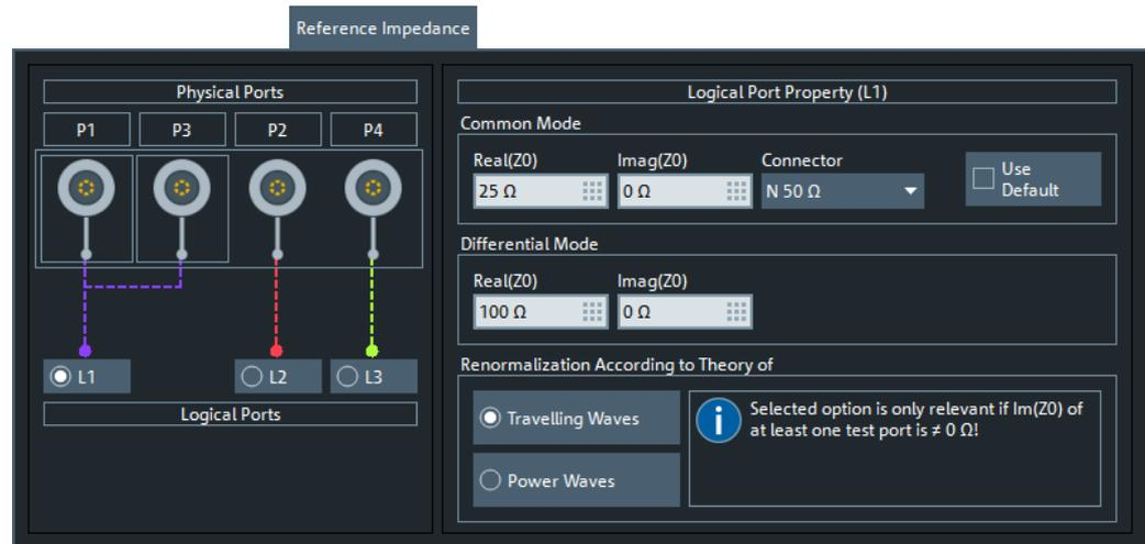
Figure 5-1: Reference Impedance Tab (4 physical ports)
