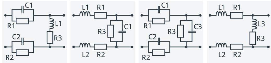
The following networks are composed of a shunt C or L (as seen from the analyzer test port), followed by two serial Cs or Ls. They are named *Shunt L*, *Serial Cs / Shunt C*, *Serial Ls / Shunt C*, *Serial Cs / Shunt L*, *Serial Ls*.
