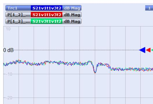
Figure 5-20: Multiple traces due to multiple paths
