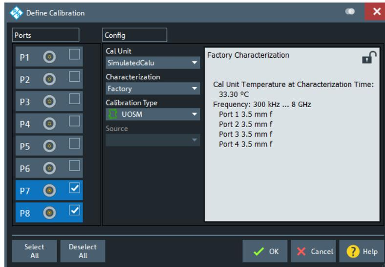
Figure 5-21: Define Calibration dialog (MultiCal, > 4 test ports)
