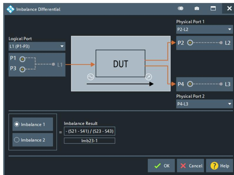
This dialog can only be opened, if a balanced and two single-ended logical ports are configured in the [Balanced Ports dialog](#).
