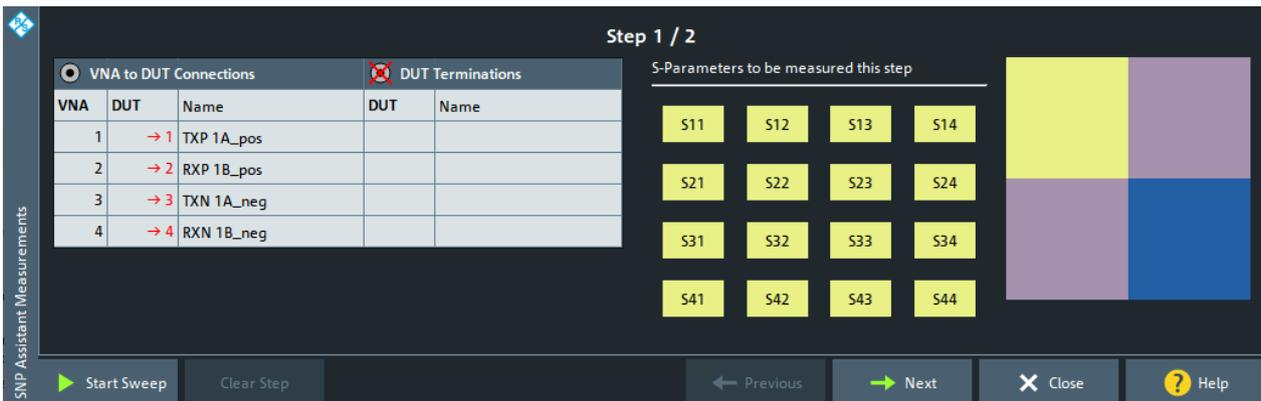
Figure 4-33: Step 3: Measure and/or import S-parameter data
