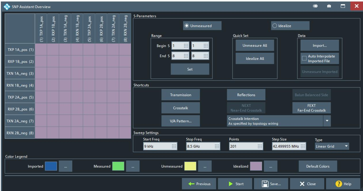
Figure 4-32: Step 2: Specify S-parameters to be measured/imported
