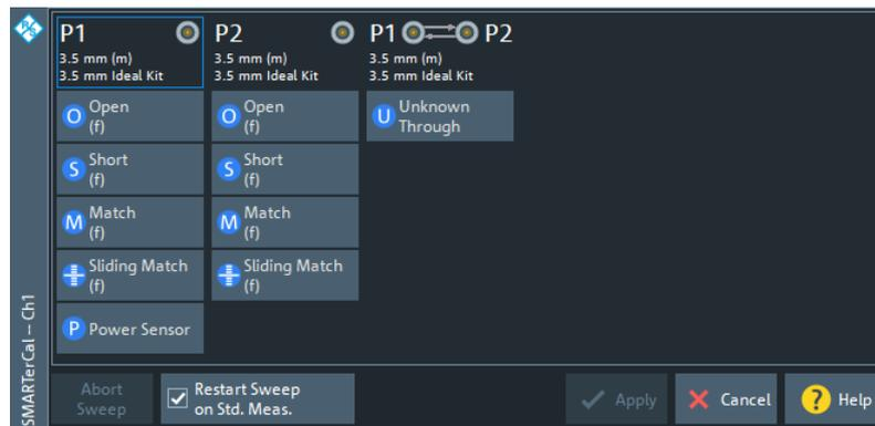
Use the buttons representing the calibration standards to start the corresponding calibration sweeps.
