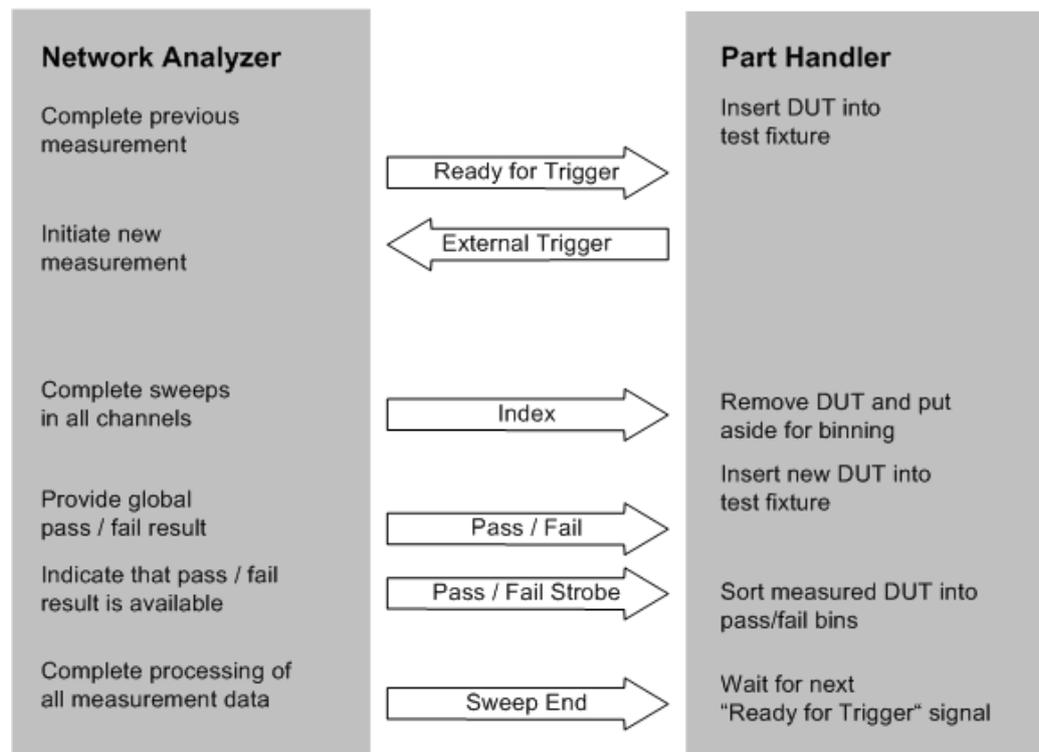
Figure 12-1: Possible stages of an automated test
