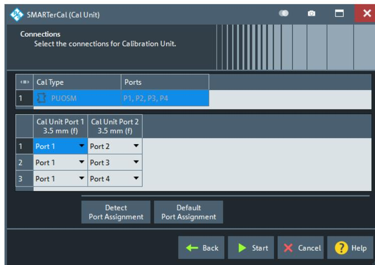
Figure 5-39: Multiple port assignments
