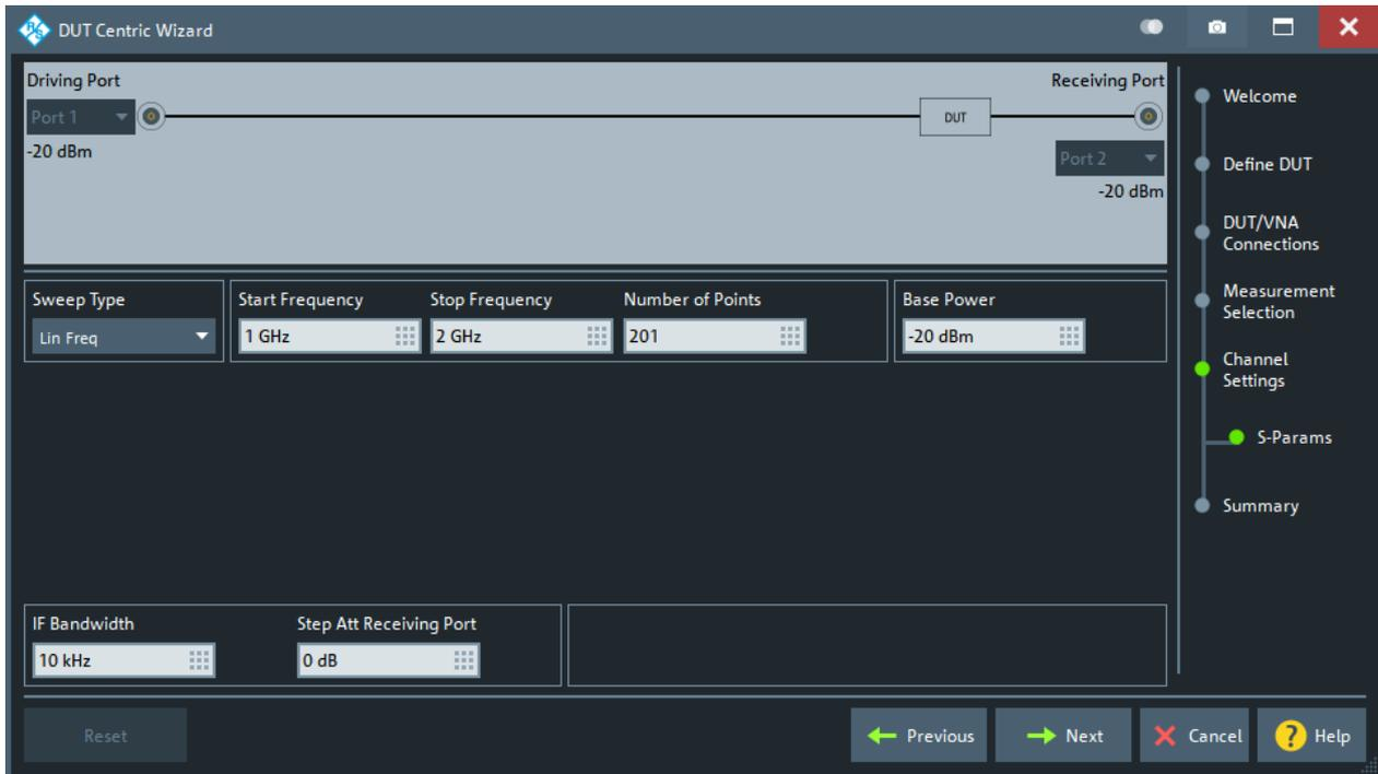
Depending on the "Measurement Selection" on page 745, either one or two channels must be set up:
