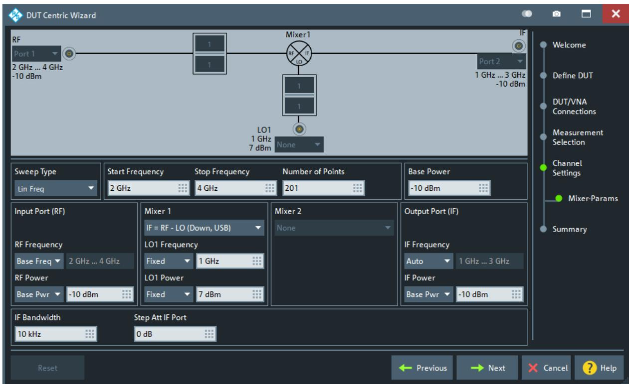
Depending on the "Measurement Selection" on page 745, either one or two channels must be set up:
