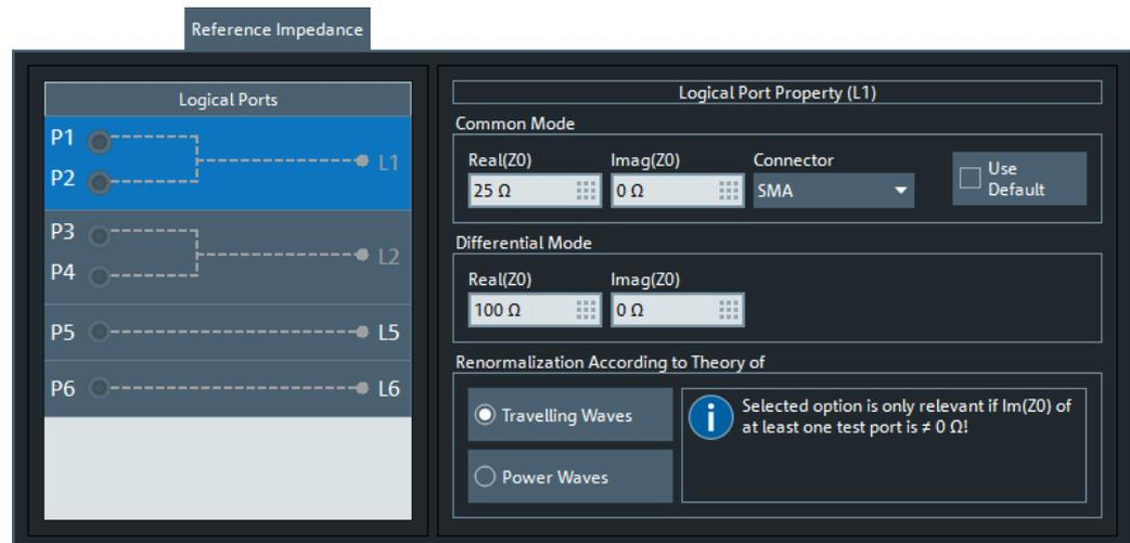
Figure 5-2: Reference Impedance Tab (>4 physical ports)
