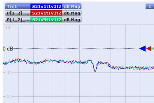
Figure 5-28: Multiple traces due to multiple paths
