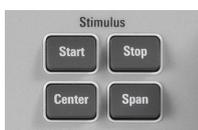
The Stimulus keys ([Start], [Stop], [Center], [Span]) define the sweep range, depending on the sweep type.
