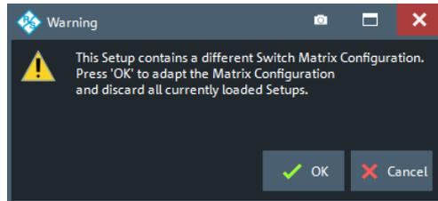
Select "Cancel" to abort the recall process or "OK" to open the [Restore Switch Matrix Configuration dialog](#) that guides you through the required configuration changes.
