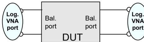
A balanced port configuration is defined in two steps: First, select the pairs of physical ports that you want to combine to form balanced ports. Second, define the two reference impedances for the differential and common mode at each balanced port. Both steps can be done in a single "Balanced Ports" dialog. The most commonly used balanced port configurations and impedances are predefined and can be selected in the "S-Parameter Wizard".
