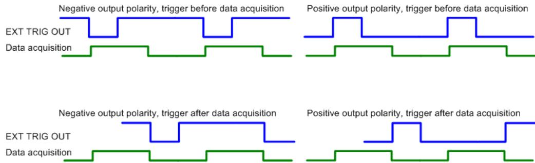
**Figure 5-11: Output trigger signal at EXT TRIG OUT**
