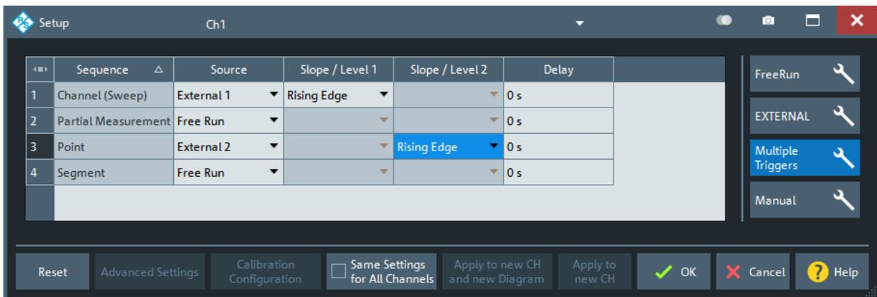
**Figure 5-10: Example of a multiple trigger configuration**
