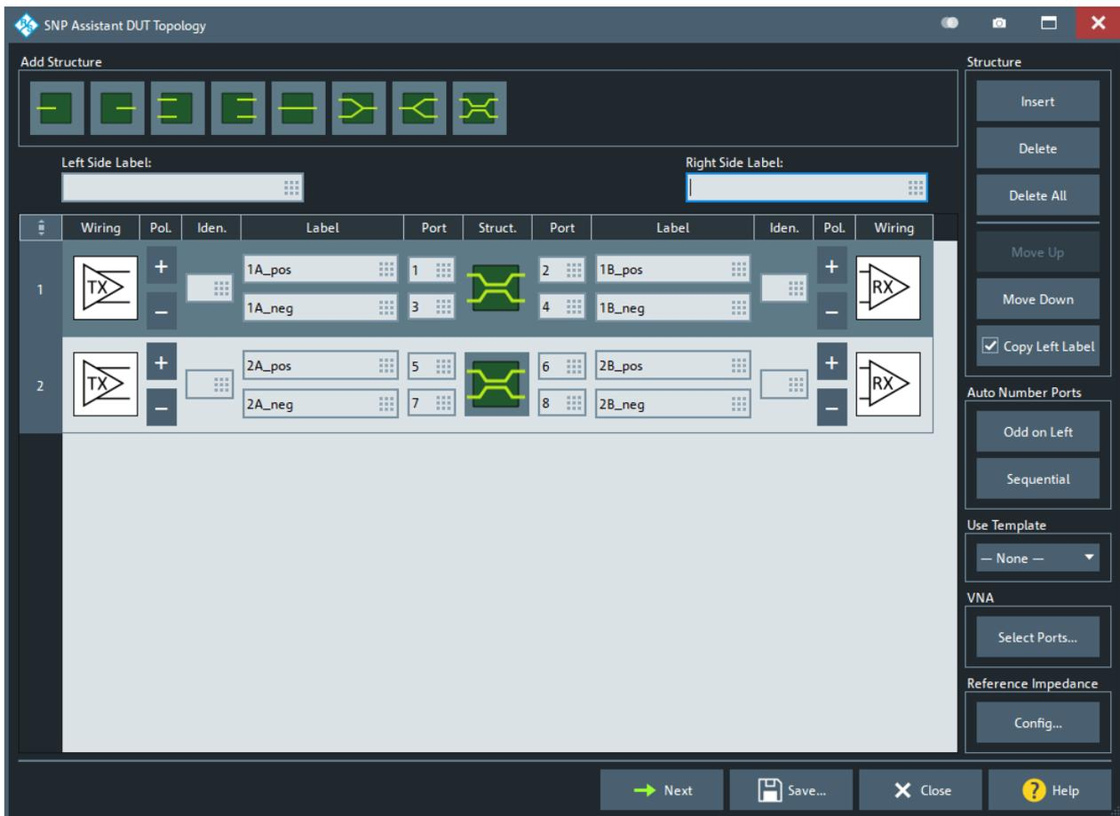
Figure 4-31: Step 1: Declare the DUT topology
