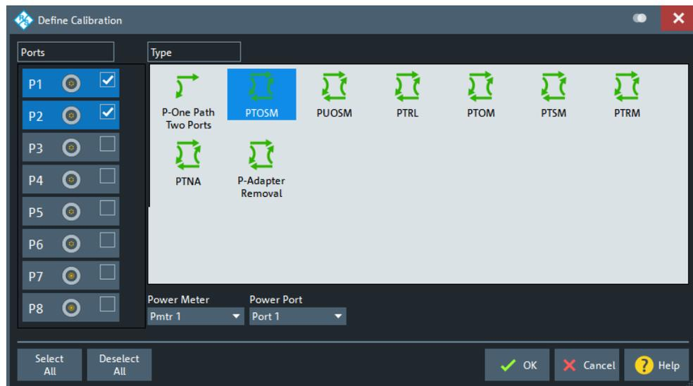
Figure 5-46: Define Calibration dialog (SMARTerCal, >4 ports)
