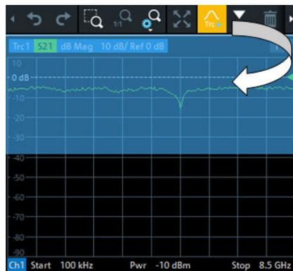
2. Select the adequate drop position, depending on whether you want to display the new trace in the existing diagram, or whether you want to add a new diagram. The highlighted area indicates the target diagram.
