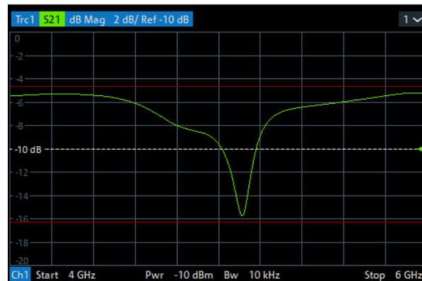
**Note:** Limit line display and limit check are independent of each other: Hiding the limit line does not switch off the limit check.
