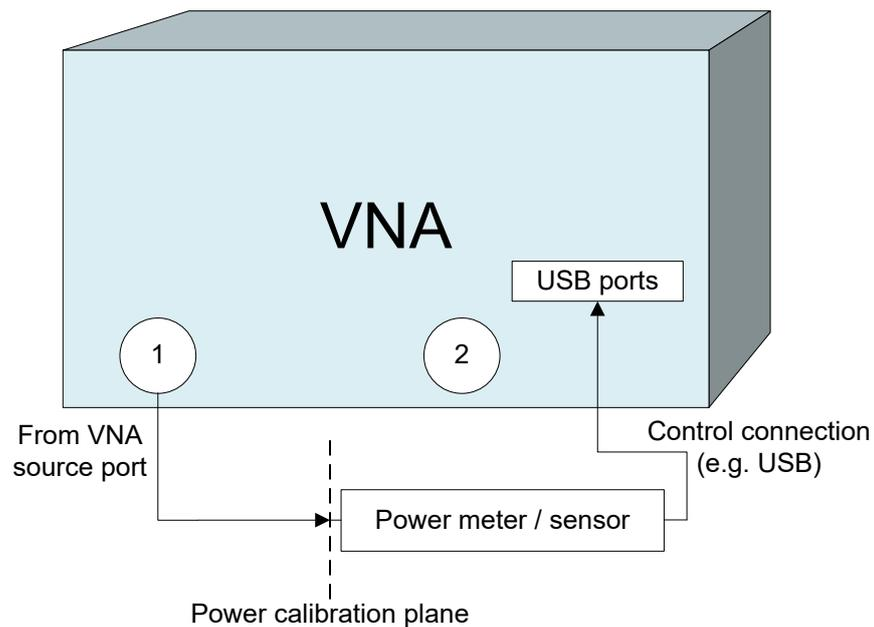
External power meters must be configured with their connection type and device address before they are available as additional receivers (System – [Setup] > "External Devices" > "Power Meters"). Configured power meters appear in many control elements of the R&S ZNB/ZNBT, e.g. in the port configuration and in the power calibration dialogs.
