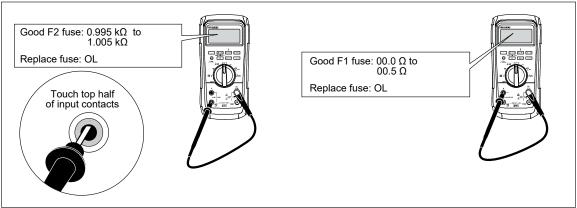
Figure 1. Current Fuse Test
