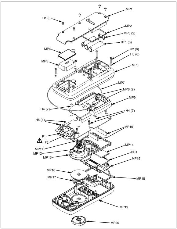
Figure 5. Exploded View of Meter
