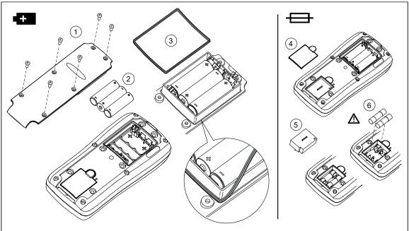
Figure 2. Battery and Fuse Replacement
