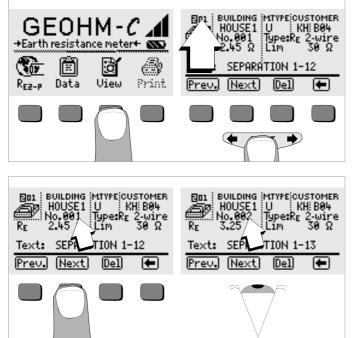
If you discover that a measurement value for the currently selected earthing system is missing, the required measurement can be performed immediately.
