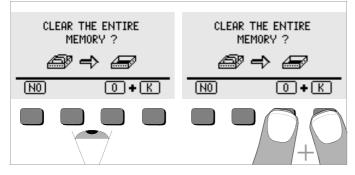
Acknowledge by simultaneously pressing O and K to delete all data from memory. The indicator to the right of the "MEMORY." parameter appears empty. Memory address "001" is displayed at the left. New data can now be entered for this address, or the database can be exited (press I or START 9 times).
