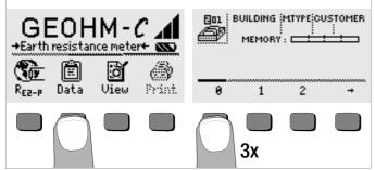
Enter memory address "000". A security request appears after acknowledgement with the START key (press at center).
