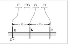
Figure 2 Measuring Earthing Resistance with a 3-Wire Test Setup
