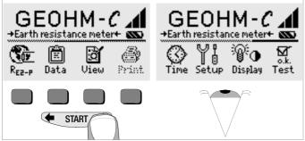
Press the  $\leftarrow$  or the  $\rightarrow$  key in order to display the desired measuring function, the desired device settings or the database functions.
