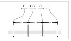
Figure 7 Measuring Soil Resistivity
