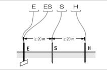
Figure 3 Measuring Earthing Resistance with a 4-Wire Test Setup
