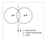
In such cases, correct measurement results can be obtained either by increasing the distance between the earth electrode and the auxiliary earth electrode, or by moving the probe along the vertical line between the earth electrode and the auxiliary earth electrode (see also Figure 5 on page 20). Moving the probe along this vertical line removes it from the zones of influence of the earth electrode and the auxiliary earth electrode.
