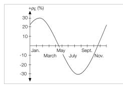
Figure 8 Soil resistivity  $\rho E$  in as influenced by season without taking precipitation into consideration (earth spike depth < 1.5 m)
