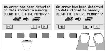
If the message shown above appears when the test instrument is switched on, you are provided with the opportunity of uploading and saving all data to a PC before deleting the memory in order to correct the error.
