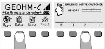
First, enter the desired memory address with the softkeys. After acknowledging this entry with the START key (press at center), the cursor appears at the first entry position (BUILDING).
