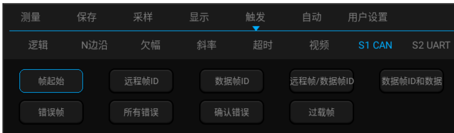
图13-15 CAN 触发方式配置菜单
