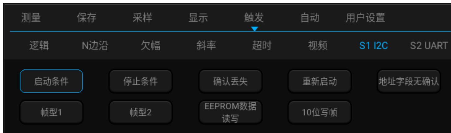
图13-23 I2C 触发方式配置菜单
