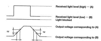
\*\* Above figure indicates that it takes 1ms per 1V to generate the voltage output corresponding to the change of received light level.
