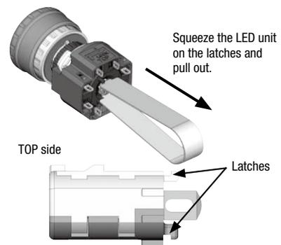
**Accessories and Replacement Parts (ø16 X6/XA Series Emergency Stop Switches)**
