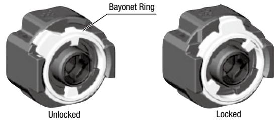
Align the small ▲ marking on the edge of the operator base with the TOP marking on the contact block. Press the contact block onto the operator and turn the contact block clockwise until the bayonet ring clicks.
