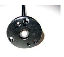
Fig. 18: Sinter filter in the sniffer handle
