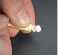
Fig. 17: Pressing the filter inserts out of the capillary filter
