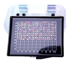
Periodically poled lithium niobate(MgO:PPLN) is a new nonlinear optical crystal. It can realize high efficiency frequency conversion of frequency doubling, sum frequency and optical parametric oscillator from visible light to mid-infrared light by (QPM) quasi-phase matching technique. Comparing with LBO and KTP, MgO:PPLN has many advantages such as high nonlinear smaller coefficient, size and shorter manufactured cycle.
