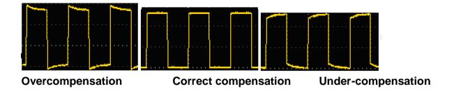
Figure 0-2: Display Waveform of Probe Compensation
