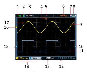
Figure 5: Oscilloscope Interface
