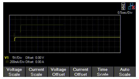
Figure 3.4 Live Output Monitoring Display
