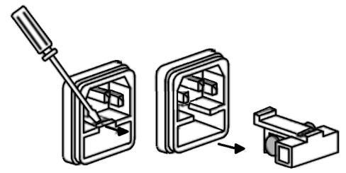
Figure 2.1 Fuse Removal
