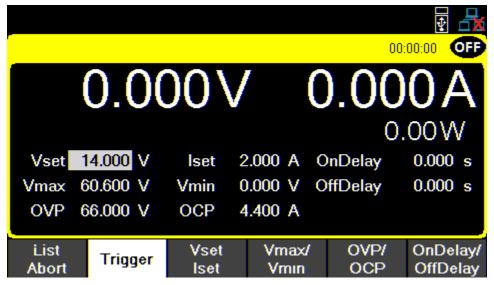
Figure 5.9 Single Channel Display Vset/Iset
