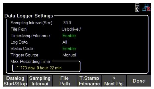
Figure 7.1 Data Logger Max Time
