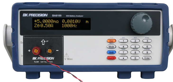
Figure 5.3 TLC81 Verification Measurement
