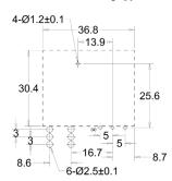
Note: In case of no tolerance shown in outline dimension: outline dimension ≤1mm, tolerance should be ±0.2mm; outline dimension >1mm and ≤5mm, tolerance should be ±0.3mm; outline dimension >5mm, tolerance should be ±0.4mm; (a) For Bi-stable 1 coil type, it is without this hole;
