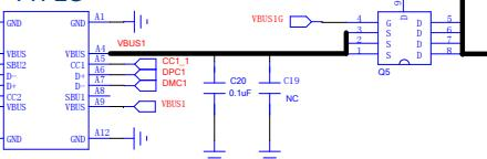
VBUS1\_I要放置在A口和C口MOS D极连接的中间节点
