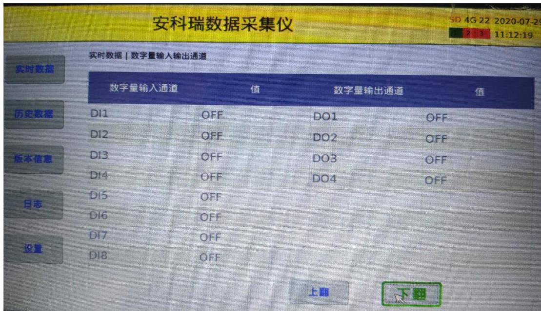
The screenshot shows the '实时数据 | 数字量输入输出通道' (Real-time Data | Digital Input/Output Channels) page. It features a table with two columns: '数字量输入通道' (Digital Input Channels) and '数字量输出通道' (Digital Output Channels). Each column has a '通道' (Channel) and a '值' (Value) column. The input channels are DI1 through DI8, and the output channels are DO1 through DO4. All values are currently 'OFF'. The page includes navigation buttons for '上翻' (Previous) and '下翻' (Next).
