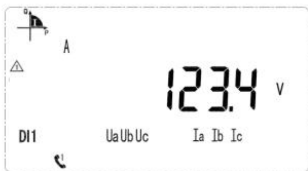
Voltage on A phase is 123.4V
