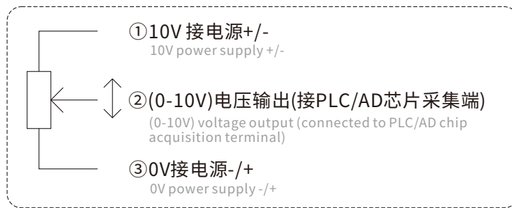
正确接线：图1 Correct wiring: Figure 1
