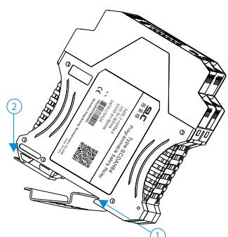
1. Insert the SCDAH84 fixed plastic clamp diagonally into one side of the installation guide rail;
